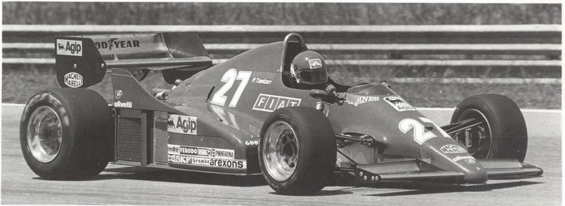
For the first races of the year Ferrari adapted the 126C2 cars to comply with the new 'flat bottom' rule. Here Tambay is at the Brazilian race in which he finished fifth.
