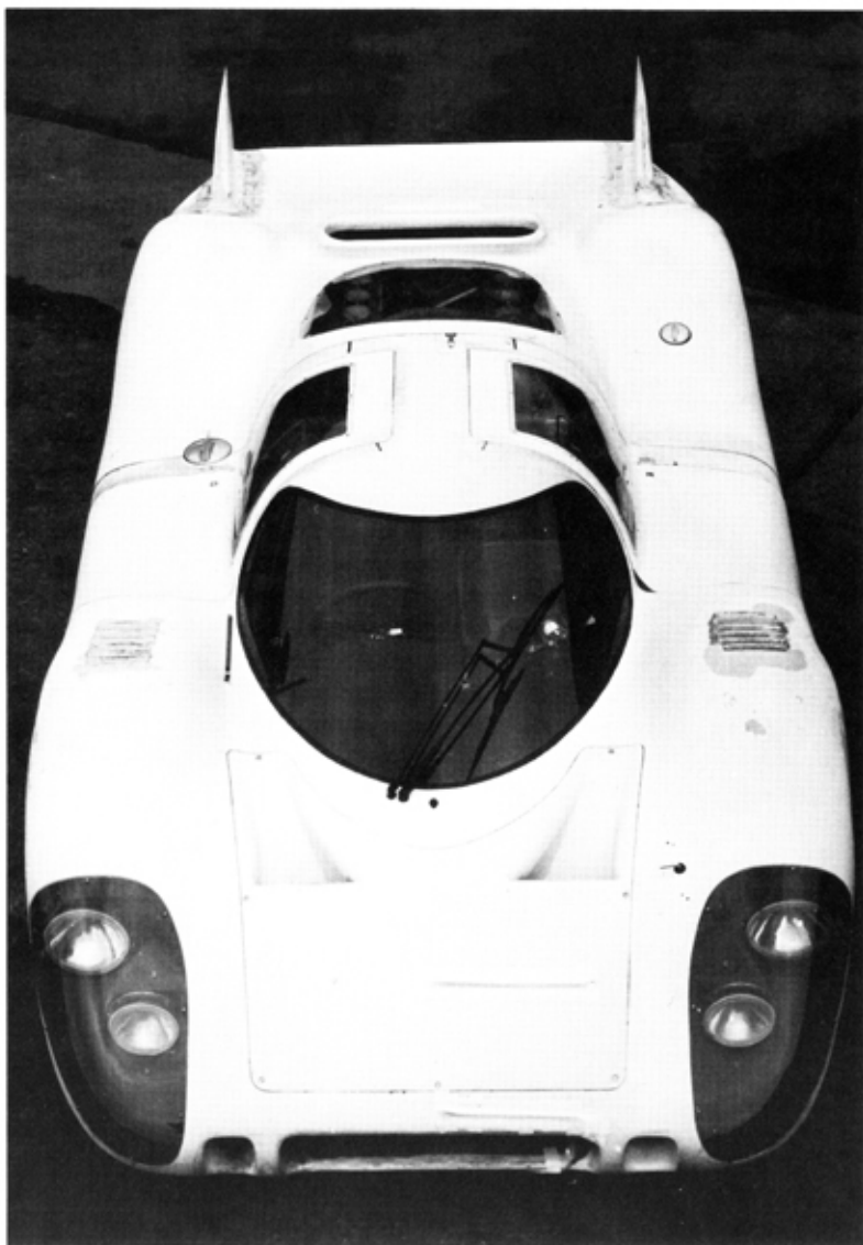
1970 Langheck from above: The new nose, the lift-measuring device beside the windshield and the hole behind the engine are apparent, as well as the test instrumentation taped to the intake.
