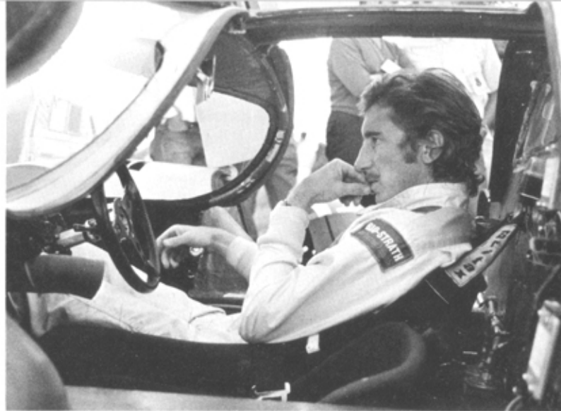
A pensive Siffert in his 917; note the reclining driving position and the tiny passenger seat.
