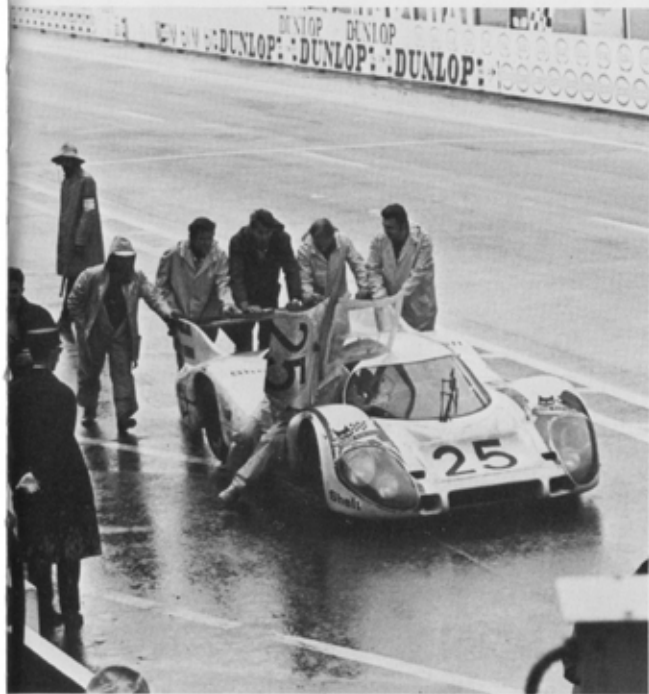
The fastest car in the race, the No.25 Salzburg 917LH led at first, was delayed with handling problems and retired after 16 hours with a broken intake valve.
