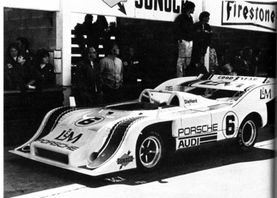
The Penske-prepared 917/10K in its finished form, with a low shovel nose and a large rear wing extending more than two feet behind the car, in the pits at Mosport. The main sponsors are Porsche/Audi and L&M, with tires from Goodyear, oil from Sunoco and battery from Sears.
