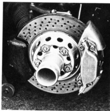
12-inch brake discs. Radial venting does not show well in 1969 photo at left; 1971 disc at right, first used at Sebring, had extensive lateral drilling to supplement radial venting.
