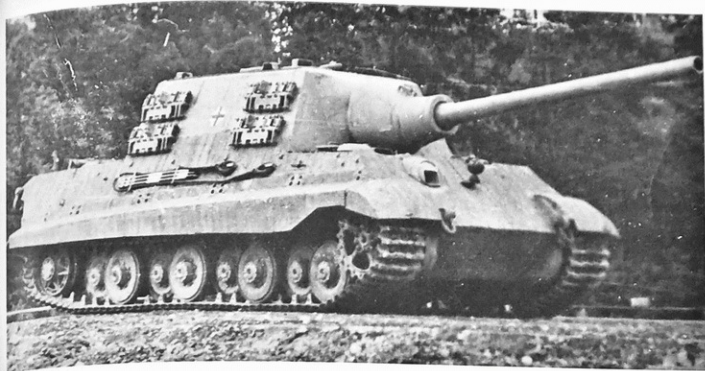
In the course of these tests, the Jagdtriger (chassis no. 305003) with Porsche running gear was fitted with Type Kps 64/640/130 tracks from the Eifelort. They did not help. The pictures show both sides, fully equipped, with spare track links on the sides of the fighting compartment. This vehicle was turned over to the Panzertruppen School in Mieland. It was the school's first Jagdtriger .
