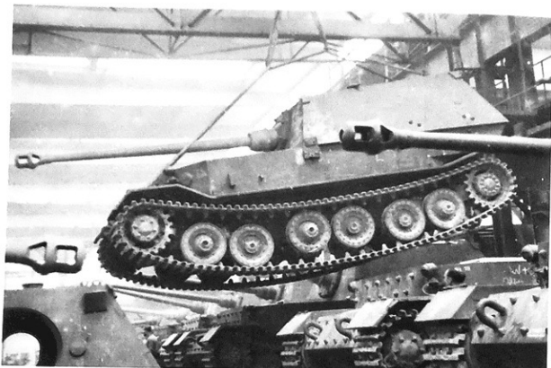
The cranes at the Nibelungenwerk were made to lift heavy loads. Thus any vehicles could be shifted without great effort and noise.
