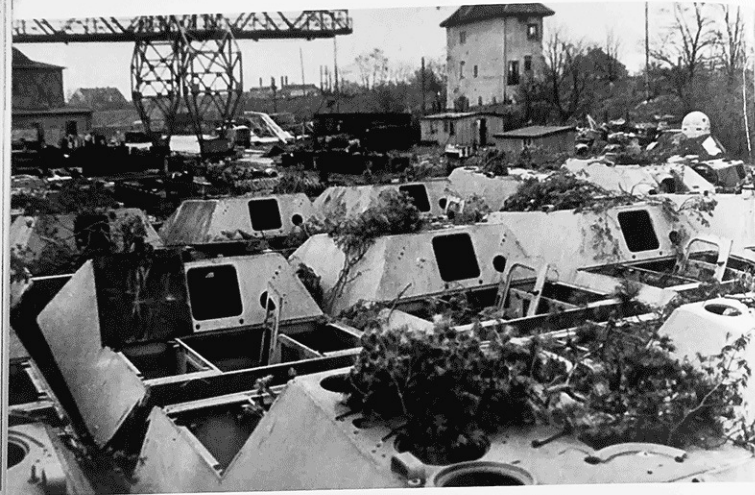
Jagdpanther bodies ready for mounting, seen at MNH at the end of the war.
