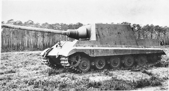
Both vehicles were tested thoroughly by the Army Ordnance Office, beginning on May 5, 1944. The Porsche running gear could not provide the required performance. Both vehicles were just painted. Zimmer was not yet applied. The racks for tools and equipment were also missing.
