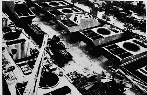
Above: The Maschinenfabrik Niedersachsen-Hanover was the only assembly firm that built Panthers and Jagdpanthers in series at the same time. The picture shows the chassis of a Type G Panther at the lower right; all those in back are Jagdpanthers. Between the two lines are engines ready for installation. Below: Two Jagdpanther bodies in the midst of Panther tank bodies, in production at MNH in April 1945.
