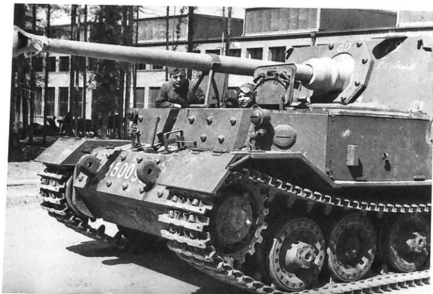
Ferdinand (chassis no. 150096) is seen after being accepted by inspectors of the Army Weapons Office. The word "Fähig" ("ready to drive") has been written on the body plate with chalk.
