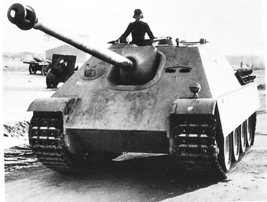
The first Jagdpanther (chassis no. V 101) was accepted by the Army Ordnance Office in October 1943. The cylindrical holder for the barrel cleaning rods on the left side is still lacking. The driver had two sight openings to use. In the sidewalls of the fighting compartment were machine-pistol loopholes. The original Type Kfg 64/660/130 still had no grippers.
