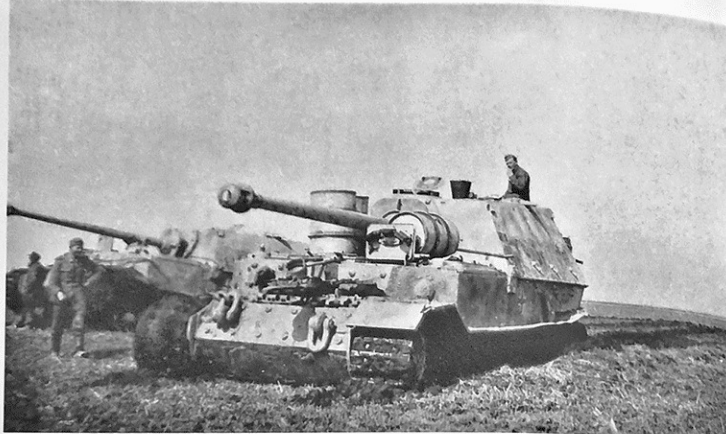
The rest of sPzJg.Abt. 653 was transferred to the eastern front at the beginning of April 1944. These two Elefant had sunk in soft ground up to their hulls before Tarnopol. The front vehicle was supplied with barrels of fuel.
