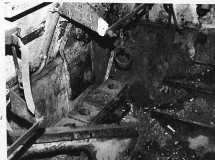
Nine racks for ammunition were located at the right rear. Part of the rack is missing.
