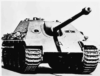
One of the first series-produced Jagdpanthers , of which MIAG produced five in January 1944. The driver's view was assured by two periscopes. The MP ports on the sidewalls were eliminated. This vehicle was sent to a Fueroerjäger replacement unit for training. Series production began with chassis no. 300001.
