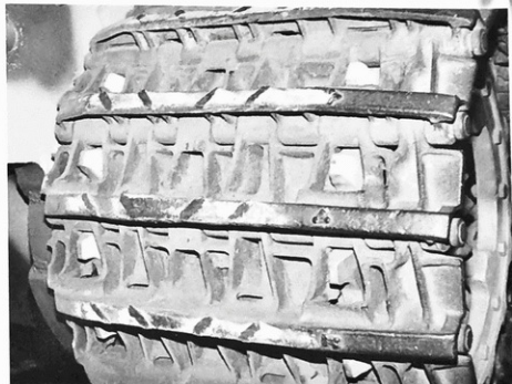
These two pictures show details of the new tracks (Type Kf 73/880/152) that were to be introduced toward the war's end for the Tiger II and Jagdiger . For these tracks, the old drive wheels with 18 teeth had to be used.
