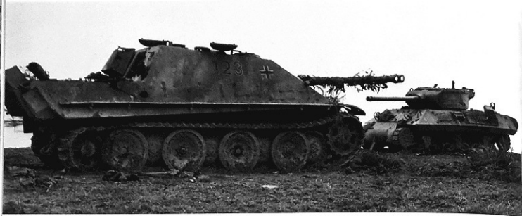
This Jagdpanther was put out of action by two KE hits in the engine compartment. In the right background is a Type M36 American tank, also shot down. This picture was taken on March 17, 1945. Until February 1945 the Jagdpanthers received a third equipment container, which was mounted on the left side of the engine compartment cover. The new leading wheels with doubled ribbing were produced sporadically from October 1944 on.
