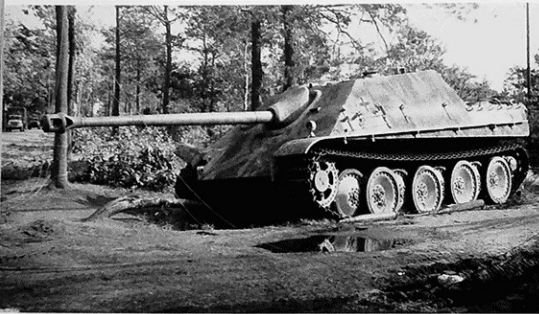
The Command Jagdpanzer, chassis no. 300054, was finished by MIAG in July 1944 and assigned to the staff of Heavy Panzerjäger Abteilung 559. Four 75 or 76 mm KE shells penetrated the rearward right side and caused a small fire in the engine compartment. The vehicle was recovered and shipped to England, where it is still on display at the Imperial War Museum.
