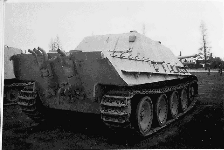
As of May 1944 two pipes were attached, one on each side of the exhaust pipe. They served to cool the exhaust temperature, and were also used to remove dust and smoke from the steering and wheel brakes.
