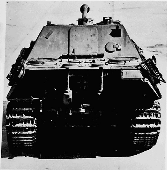
The towing shackle attached to the center of the rear plate was formerly welded to the round servicing hatch. In recovery, towing rods could now be used. To make place for the new towing coupling the winch, formerly mounted horizontally, had to be placed vertically between the exhaust mufflers. The vehicle shown is a command tank, with a mount for a star antenna on the upper right part of the rear wall.
