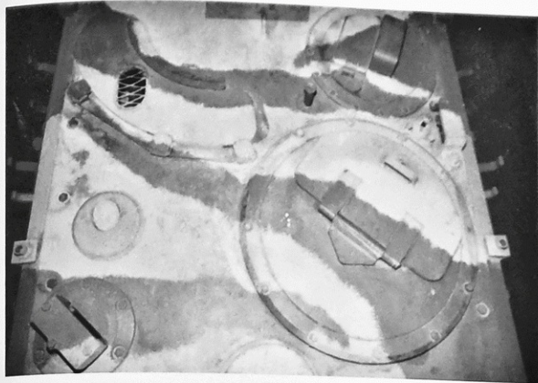
The roof of the Jagdtiger fighting compartment. The bolt in front of the commander's hatch is an attachment for the planned range finder.
