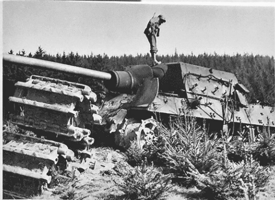
One of the last Jagdtiger, made in February or March 1945 and turned over to s.Pz.Jg.Abt. 512. The vehicle has the four "mushrooms" for attaching the two-ton crane. The vehicle was hit several times by KE shells, or the tracks were damaged and finally blown up by the crew.
