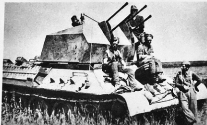
The unusual equipment included a 2 cm Flak quad on the chassis of a Russian T 34.
