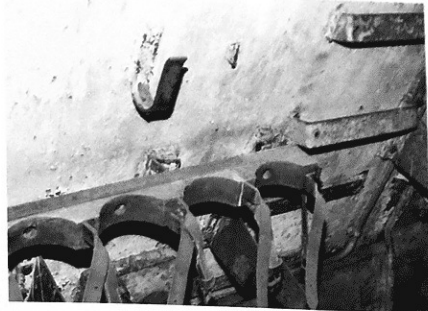
Racks for six shells on the right side of the fighting compartment.
