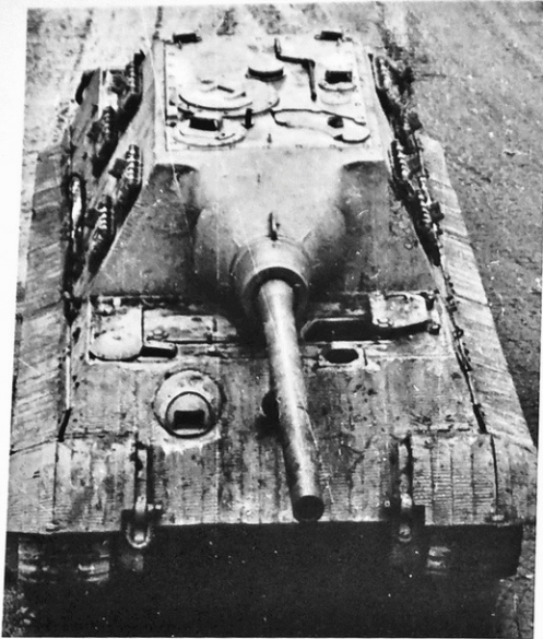
A front view of the vehicle, seen from above. The driver's hatch is open. The paint is dark yellow, with RAL shade 7028. The "Zimmerit" coating was applied only as high up as a man could reach.
