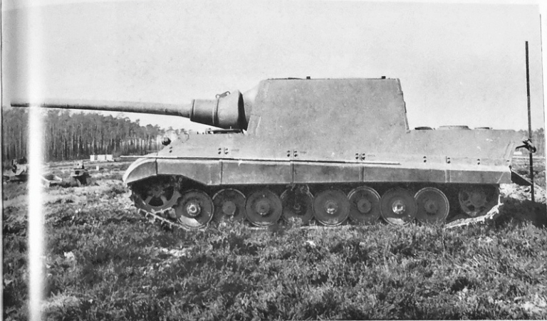
The first two Jagdtiger were finished in February 1944. The first vehicle (chassis no. 305001) was built with the Porsche running gear of eight road wheels (700 mm diameter) on each side.
