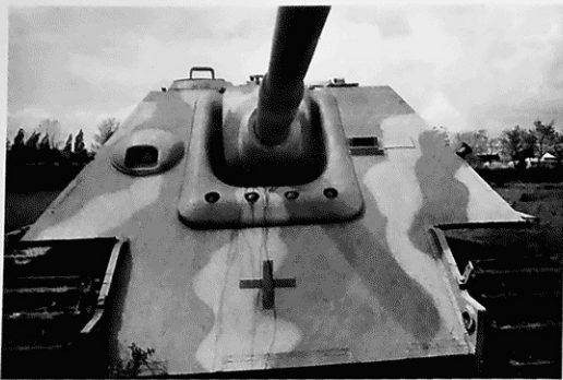
In February 1944 production the left periscope for the driver was eliminated. The opening was covered by a welded on rectangular plate.
