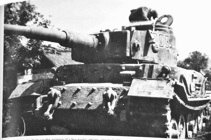
Noteworthy in this structure was the assigning of a few exotic vehicles, almost all of them one-offs. These vehicles were to be found in the Abteilung Staff, Gruppe Führer. This Tiger (P) (VK 4501(P)) was used as a command tank, its commander being Captain Hanns Wegelin. The tactical number was 003. The picture shows the front of the Tiger reinforced with added armor plates.
