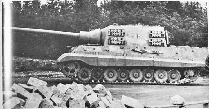
Both vehicles were tested thoroughly by the Army Ordnance Office, beginning on May 5, 1944. The Porsche running gear could not provide the required performance. Both vehicles were just painted. Zimmer was not yet applied. The racks for tools and equipment were also missing.
