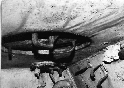
The loader's entry-exit hatch was at the left rear of the roof. Behind it, in the far corner of the fighting compartment, was the periscope mount.
