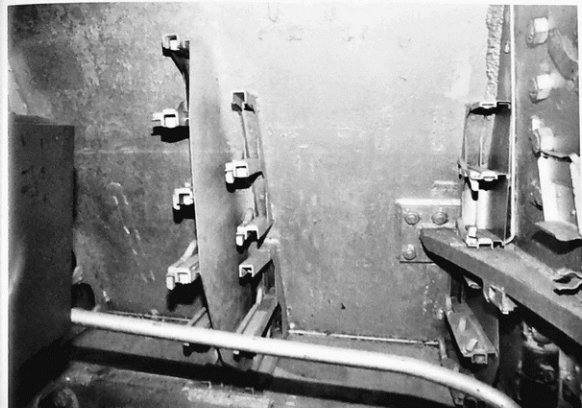
Left side: The commander's battle station and the racks for 6 + 8 cartridges.
