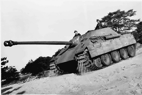
After the early Jagdpanthers had been equipped with a single-piece barrel for the 8.8 cm Pak 43/3, a version of this weapon with a two-piece barrel was used as of May 1944. All the supplies were used up, so that by the end of October 1944, Jagdpanthers with the one-piece barrel were still delivered. The one-piece barrel is shown above, the two-piece type below. (BA, BA)
