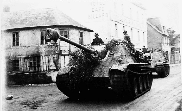
The Jagdpanther in action in France, 1944. The small ball mantlet and the left opening for the driver's periscope, now welded shut, can be seen clearly. (BA)
