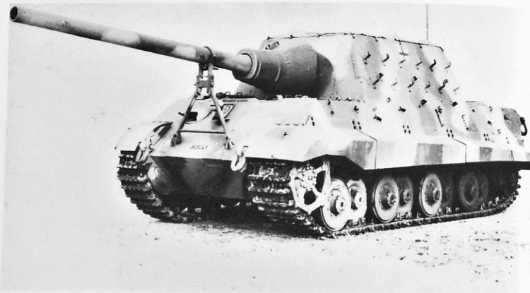
The first Jagdtiger with Porsche running gear (chassis no. 305001) was reequipped by Verskraft in Kummersdorf. Now twelve hooks for spare track links are welded onto each side of the fighting compartment. A barrel brace for the cannon was mounted on the upper bow plate.
