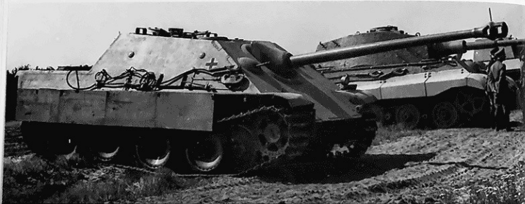
The second prototype was shown to Hitler on December 16, 1943. The two machine-pistol ports can be seen on the right wall of the fighting compartment. They allowed use of MP for close range defense, and for observation. In the background is a Tiger H 2 tank.
