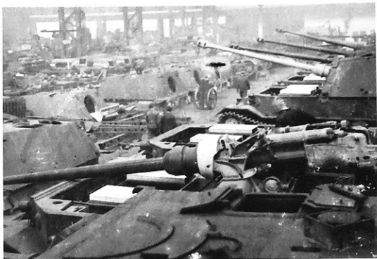
This picture from above shows the rectangular hatch for the commander. The rear lid had to be opened all the way when the commander wanted to use his shear scope. The nearest vehicle affords a rare view of details of weapon installation.
