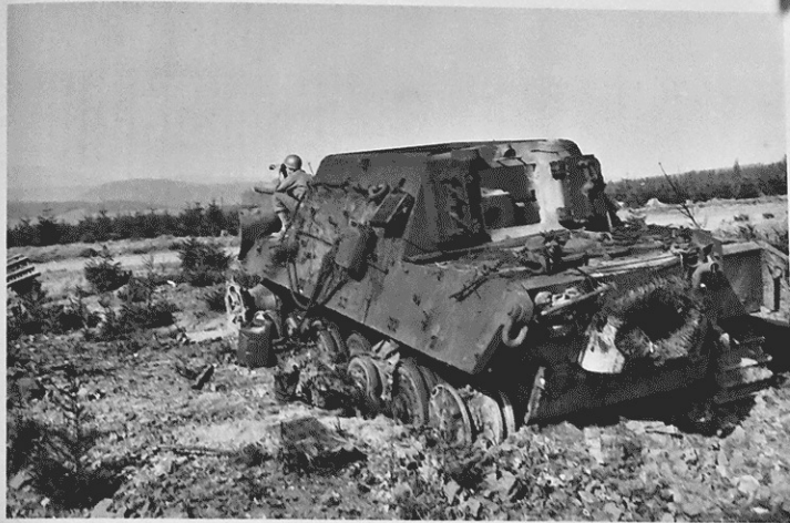
This picture, taken on 4/16/1945, seems to attest to the rumor that track supplies were not assured. The Type Cg 24/660/300 tracks of this vehicle were loading tracks for railroad transport; they were not to be used offroad. The ground pressure was much too high.
