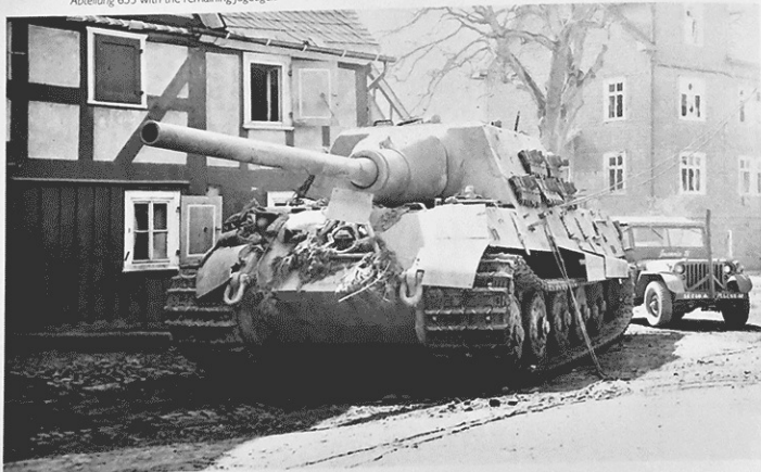
This Jagdtiger (chassis no. 3050580) was finished in January 1945, and sent to Heavy Panzerjäger Abteilung 653 in March 1945. Captured by the US Army in Germany, the vehicle shows the six sets of spare track links attached at the factory since December 1944. The driver's and radoman's hatches each had two handholds.
