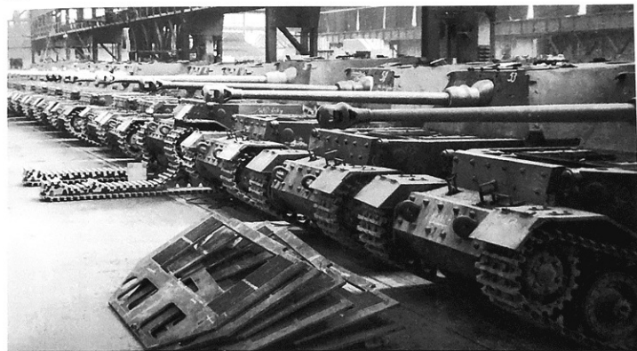
Almost finished Ferdinands. The covering of the driver's space must be attached. Chassis no. 150027 is first in line at right.
