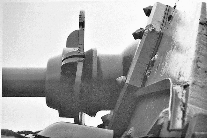
The Ferdinands left the factory with unprotected ball mantlets. Krupp of Essen sent the additional armor to the troops by rail on May 13, 1943. The troops mounted them themselves before going into action.
