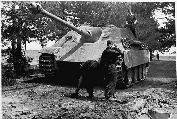
After the early Jagdpanthers had been equipped with a single-piece barrel for the 8.8 cm Pak 43/3, a version of this weapon with a two-piece barrel was used as of May 1944. All the supplies were used up, so that by the end of October 1944, Jagdpanthers with the one-piece barrel were still delivered. The one-piece barrel is shown above, the two-piece type below. (BA, BA)
