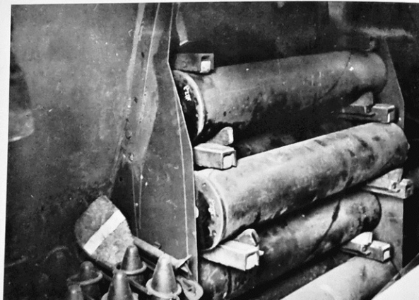
Storage of the separated ammunition, cartridges lying, shells standing (chassis no. 305058).
