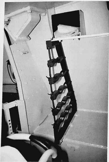
The rear body wall with the square entrance-exit hatch. To the left is a round port for throwing out used cartridges.
