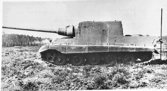
The second vehicle, which was produced at the same time (chassis no. 305002) had the Henschel running gear with nine road wheels (600 mm diameter) on each side.
