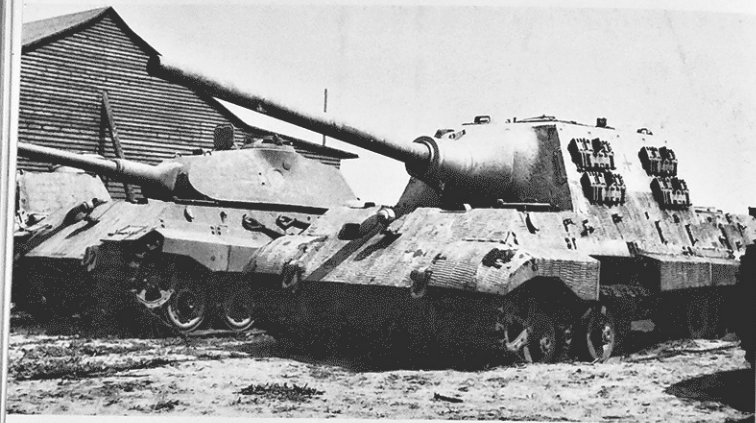
The Jagdiger (chassis no. 305004) was also sent to the proving grounds of the Army Ordnance Office, and was captured by British troops at a training camp. It was sent to Bovington, where it is still to be seen in the museum. The barrel brace was not yet installed, and the third wheel track of the Porsche running gear is missing. It broke off during driving tests. Next to it is a Tiger tank, Type B, with the early turret.
