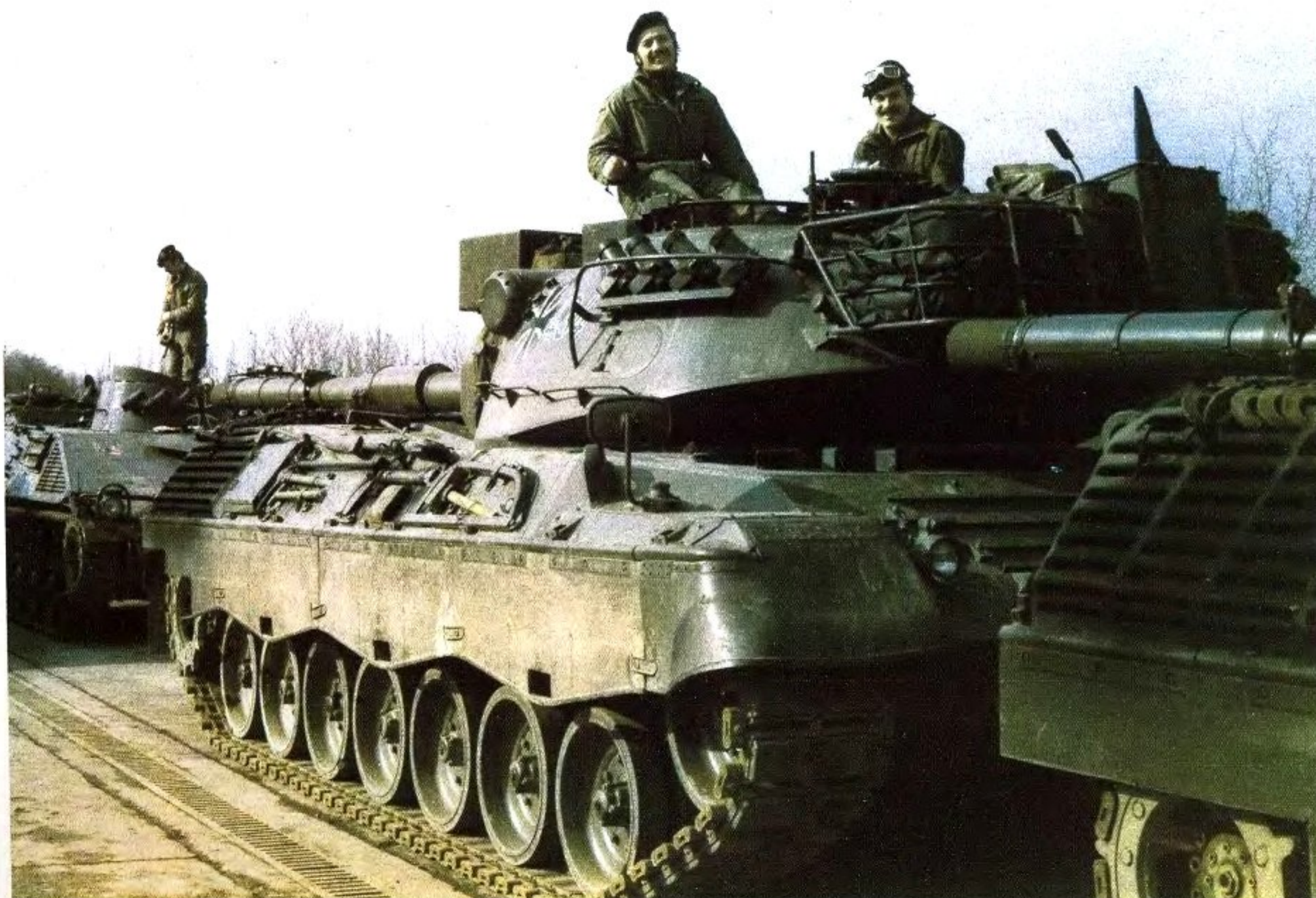
Leopard A1 MBTs of different batches loaded on railway platform cars in July 1976. The wooden wedges used to fasten the tanks to the cars have already been removed. In 1976, the fitting of add-on armour to Leopard A1 tanks was in progress. The 2 nd Company of the 202 nd Tank Battalion was already equipped with a few of these upgraded A1A1 vehicles as seen here with the fourth vehicle for exercise at the NATO training area of Bergen. (JP)
