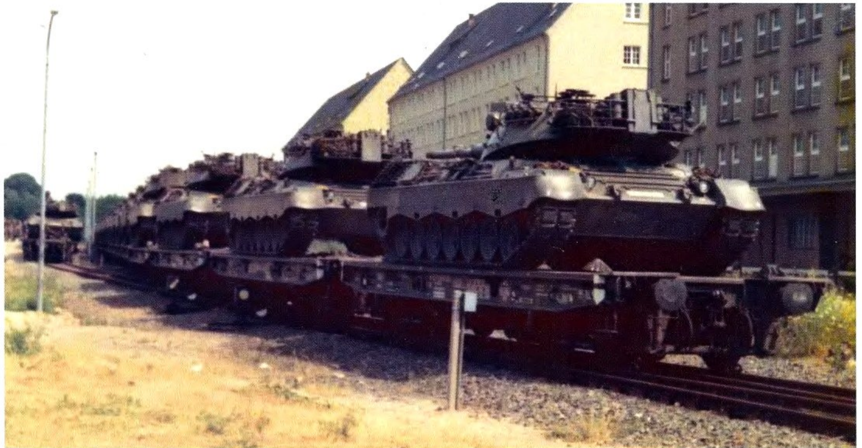
Leopard A1 MBTs of different batches loaded on railway platform cars in July 1976. The wooden wedges used to fasten the tanks to the cars have already been removed. In 1976, the fitting of add-on armour to Leopard A1 tanks was in progress. The 2 nd Company of the 202 nd Tank Battalion was already equipped with a few of these upgraded A1A1 vehicles as seen here with the fourth vehicle for exercise at the NATO training area of Bergen. (JP)
