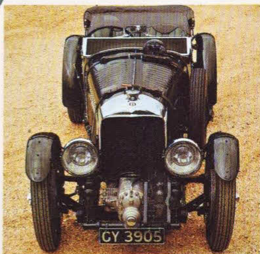
Amherst Villiers' supercharger on the nose typified the 1930-31 'Blower' Bentley.
