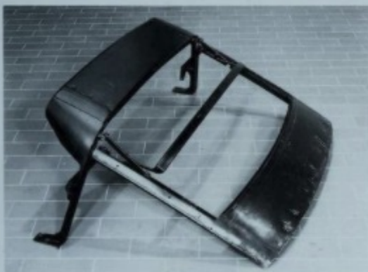
New benchmarks. About half of the 911 top consists of stamped steel panels.
