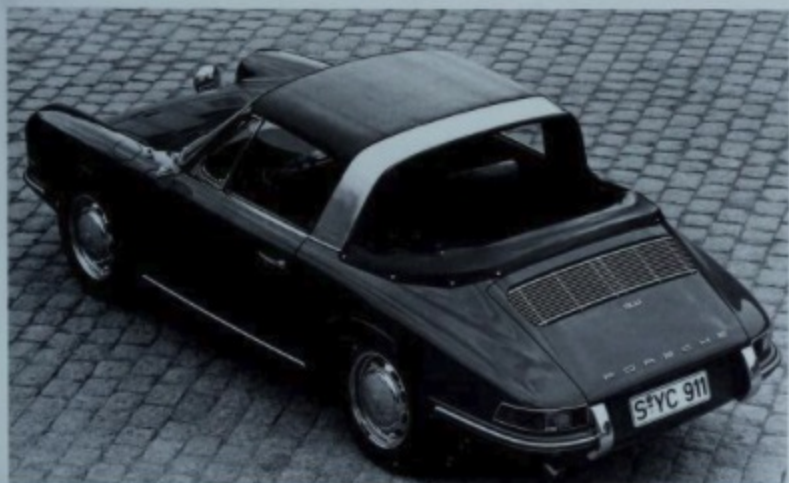
Targa Voyage. Folding top and the rear window can be removed by means of a single zipper.
