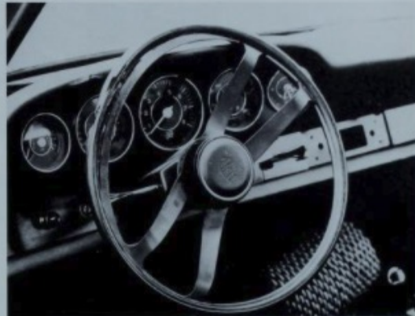
Danger: the wood-rimmed steering wheels which were standard equipment in the first model year could splinter as a result of an accident.
