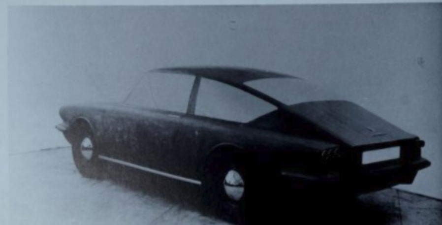
...yet a full-scale, three-ton clay model was made.
