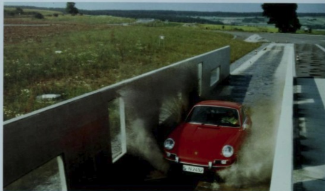
Porsche has had a test track at Weissach since 1969. The 911 shown here is driving through a salt water bath, part of an endurance test.
