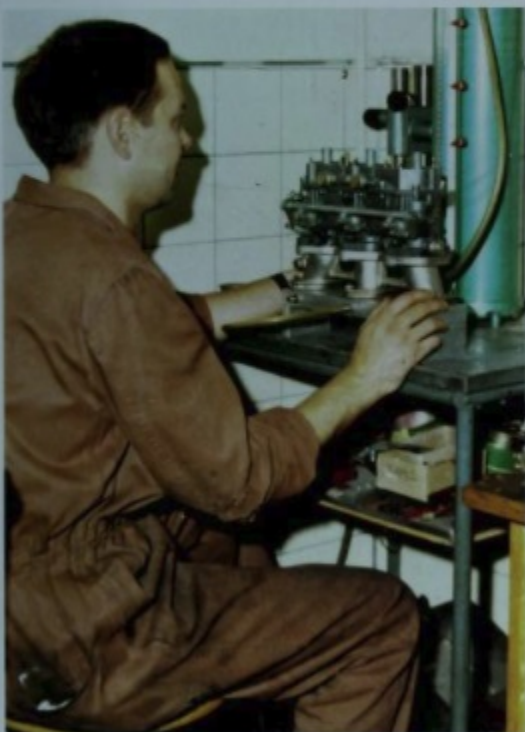
Carburetor banks were carefully checked before installation.
