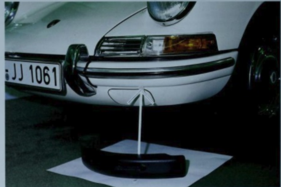
These cast iron bumper reinforcements were installed in production cars beginning with serial number 301340.
