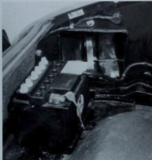
For improved weight distribution, batteries were located in the left and right front fenders.
