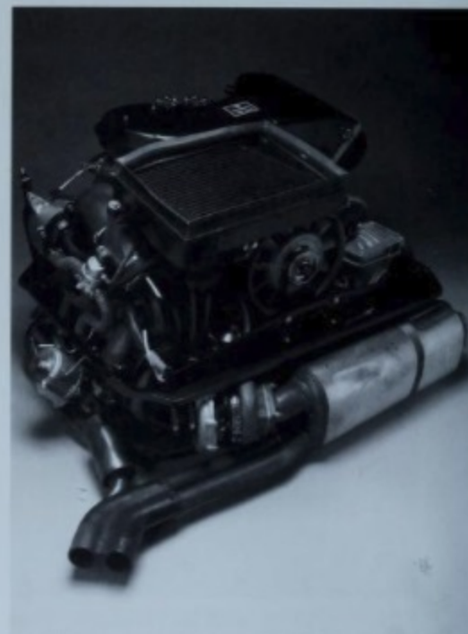
The 300-horsepower 3.3-liter engine is recognizable by its large intercooler.
