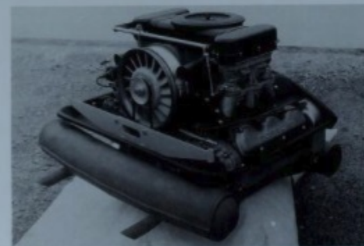
The engine shown here, with two single overhead cams, was built in 1963 and served in a 901 prototype. For production, the air filters and the muffler were changed.
