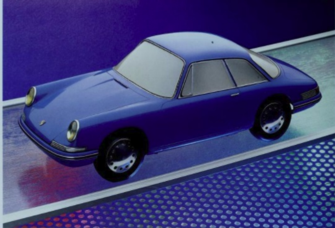
The first Plasticine model of the Type 754 T7 was completed on October 9, 1959. This cast resin copy was pulled from the clay and given a fresh coat of blue paint.
