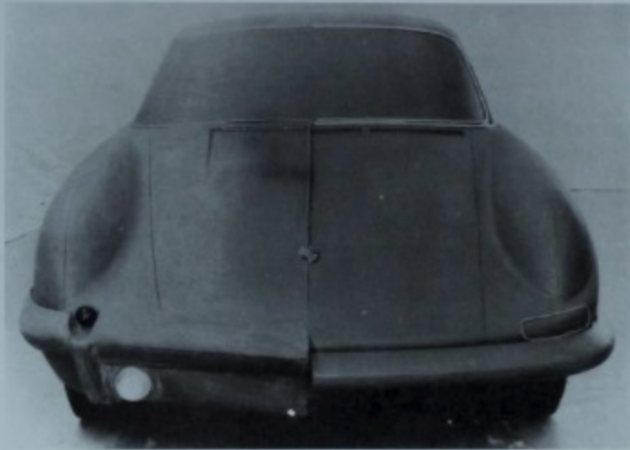
The left half of the Plasticine model was developed by the Porsche model department under Heinrich Klie; the right side is a Count Goertz design.
