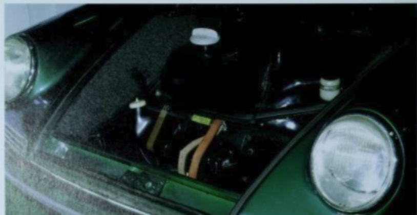
For refueling, the trunklid had to be opened. The fuel filler lid on the left front fender would come later.
