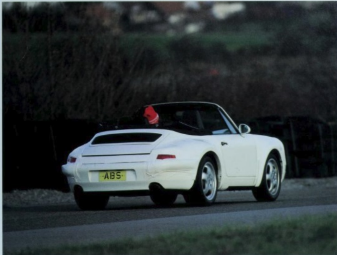
November 1992, at the Weissach proving grounds. Even in the depths of winter, Cabriolets must cover 3000 km, half of the test distance, with the top down.
