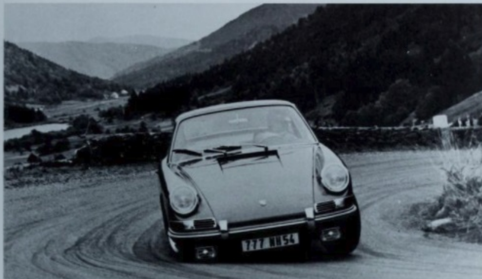
The first 911s, without stabilizer bars, showed excessive lean in corners. At the limit of adhesion, the unloaded front tire provided no steering forces.
