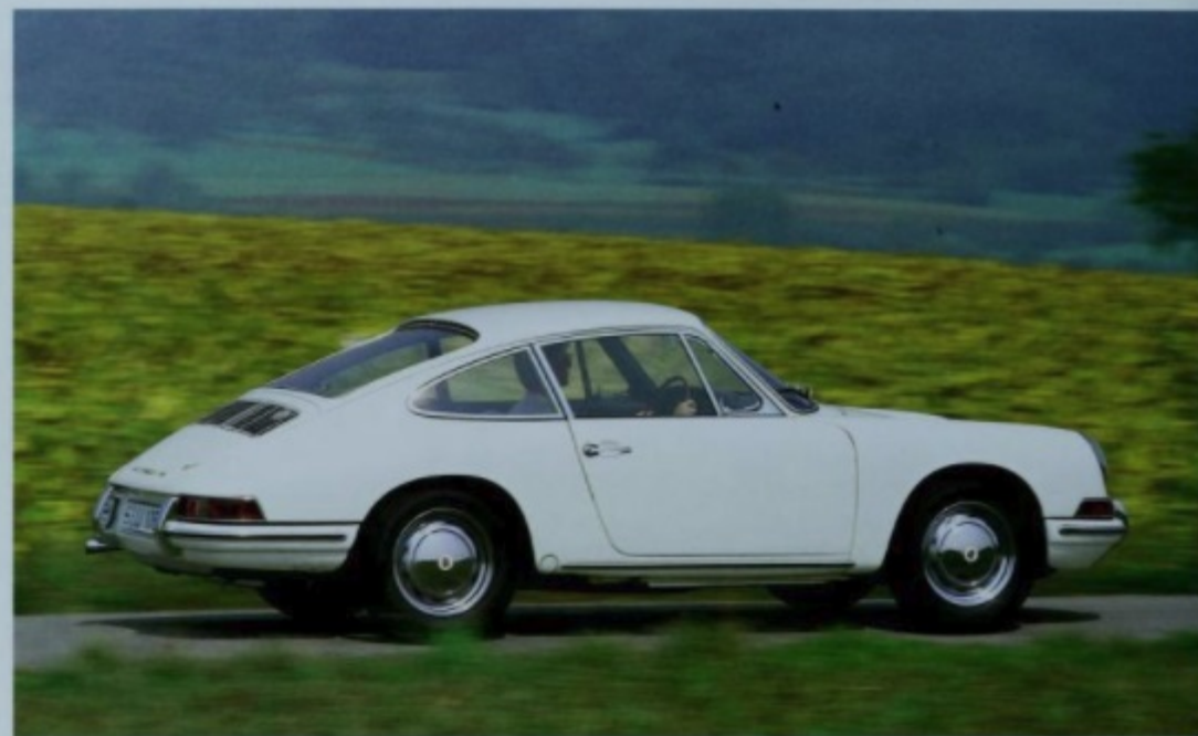
Due to their rearward weight distribution, the first 911s had a basic oversteering tendency, poor straight-line stability and high crosswind sensitivity.
