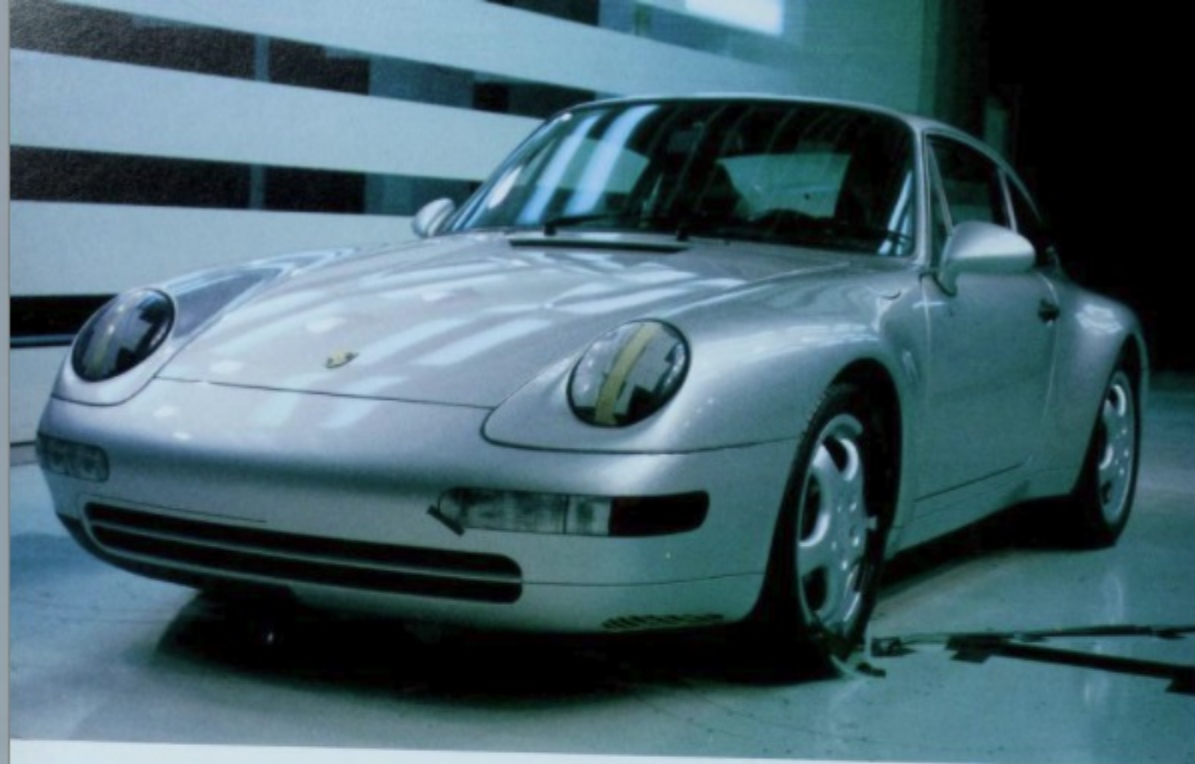
The final stage of Project 993, undergoing wind tunnel testing. Headlights and wheels do not represent production pieces.
