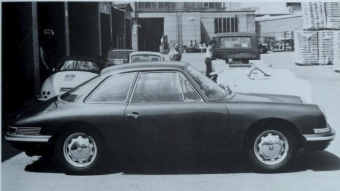
Type 754 T7: The roofline sloped gently downward, with a slight break...
