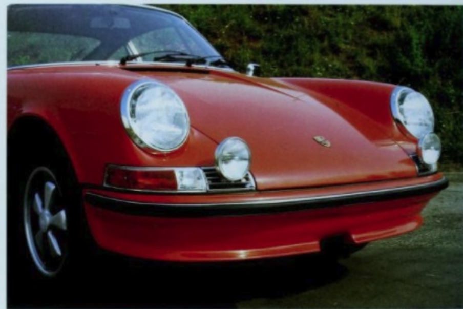
Beginning with the 1972 model year, the S models were fitted with a front air dam to reduce lift.
