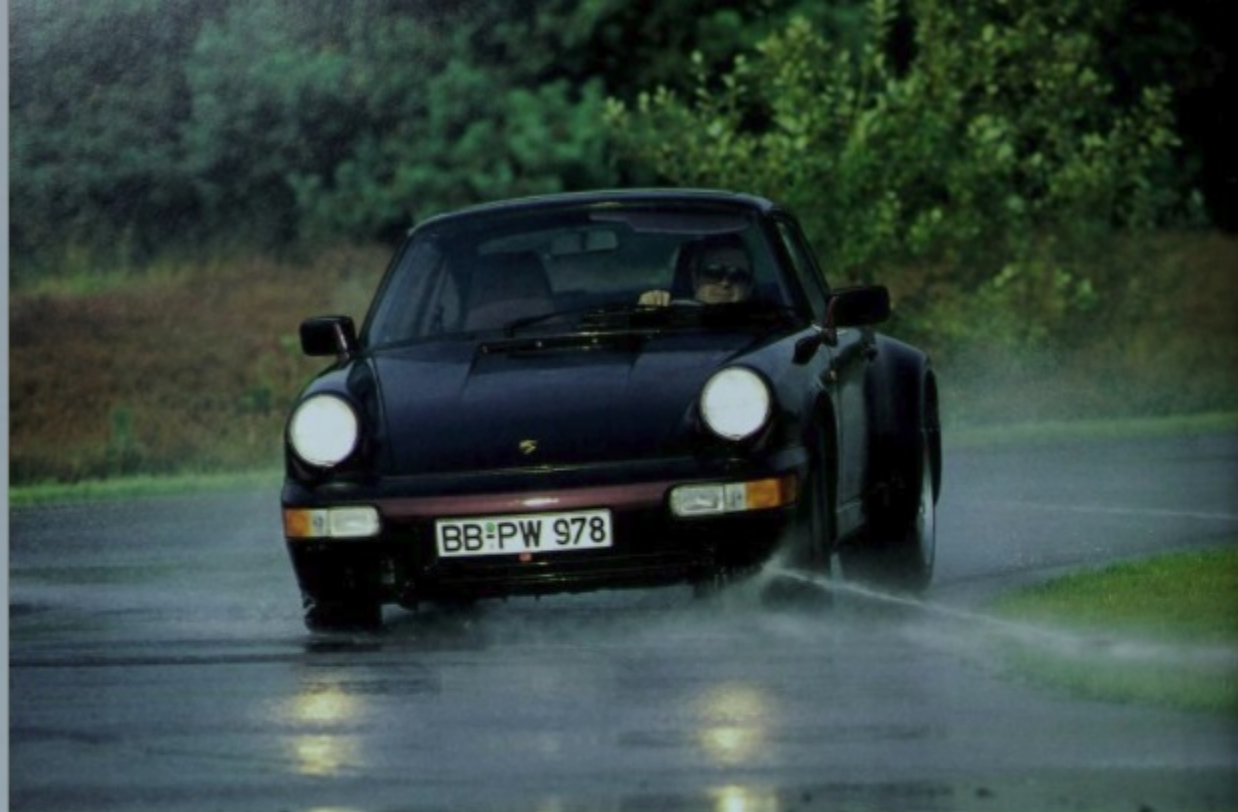
September, 1991: wet handling tests at the Contidrom. This Type 964 Carrera, with the narrow front and wide rear track of the Turbo-look package, is powered by an early version of the 993 powerplant.
