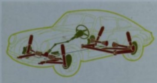
Phantom drawing of the 911 suspension, showing the safety steering column.
