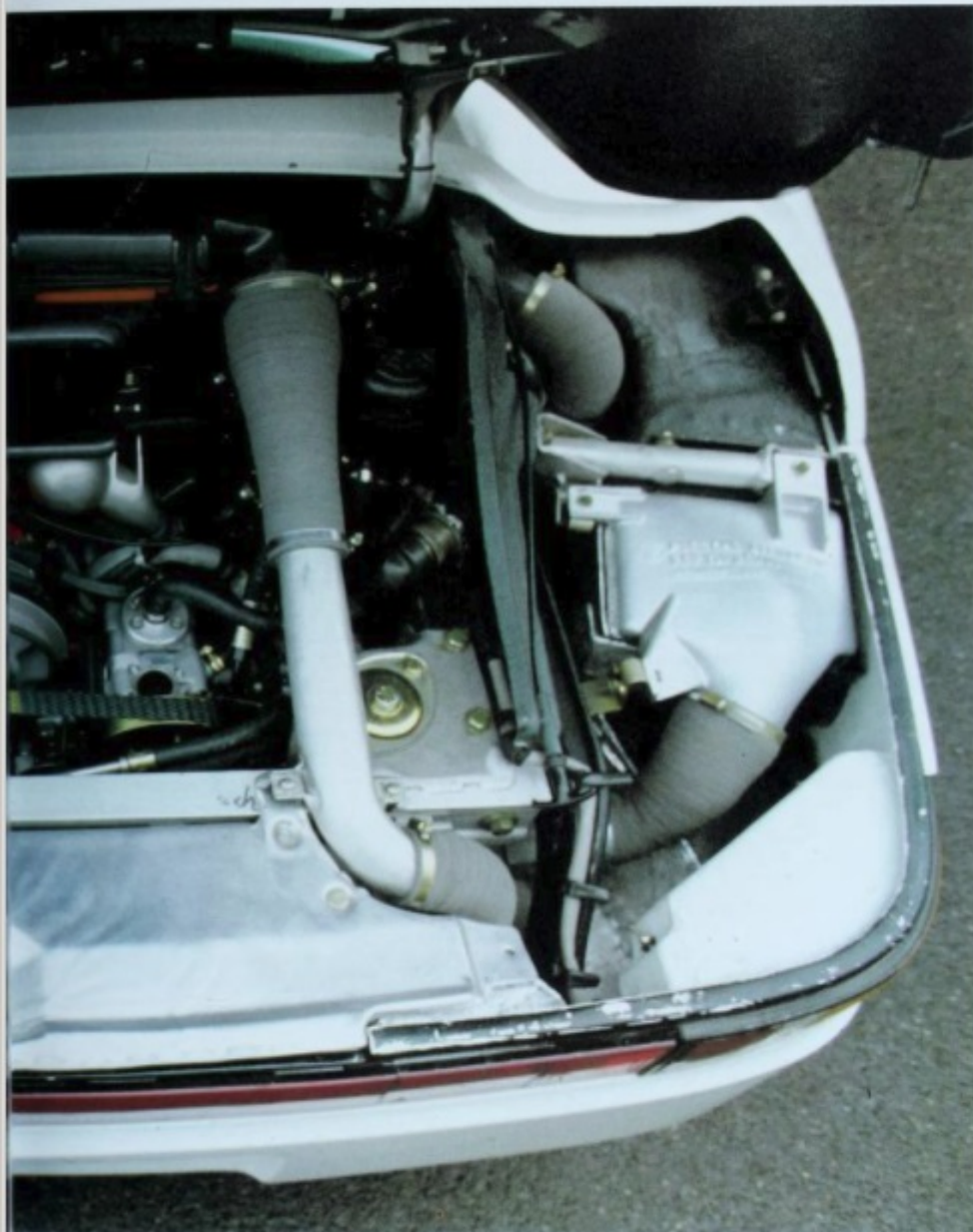
The most exciting powerplant ever installed in a roadgoing Porsche. It squeezes 450 horsepower out of only 2.85 liters.
