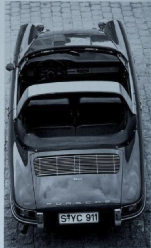
Targa Spyder. Without roof panel and with folded rear window, Targas offered virtually all the pleasures of a full convertible.
