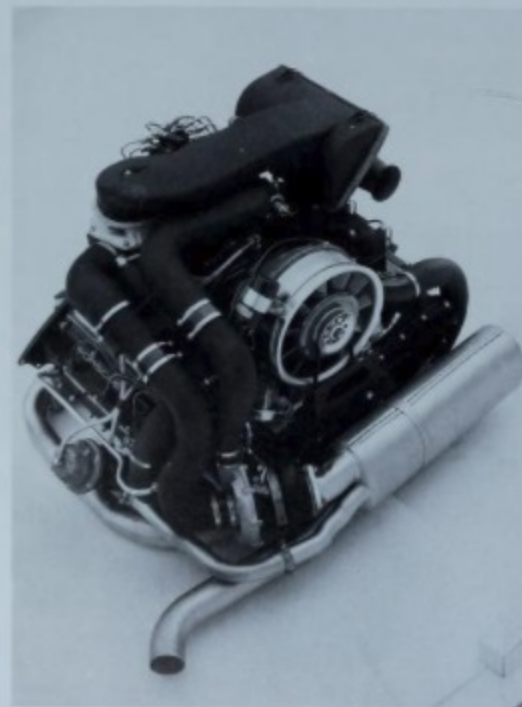
The engine of the three-liter 911 Turbo was based on the normally-aspirated engine of the Carrera 3.0.
