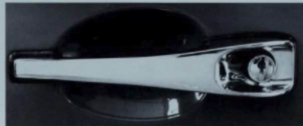
The recessed pushbutton prevents the door from opening during a rollover accident.
