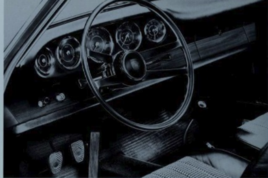
The cockpit of the first production cars, with a wood-rimmed steering wheel and wooden dash trim. The configuration of five round instruments has been retained to the present day.
