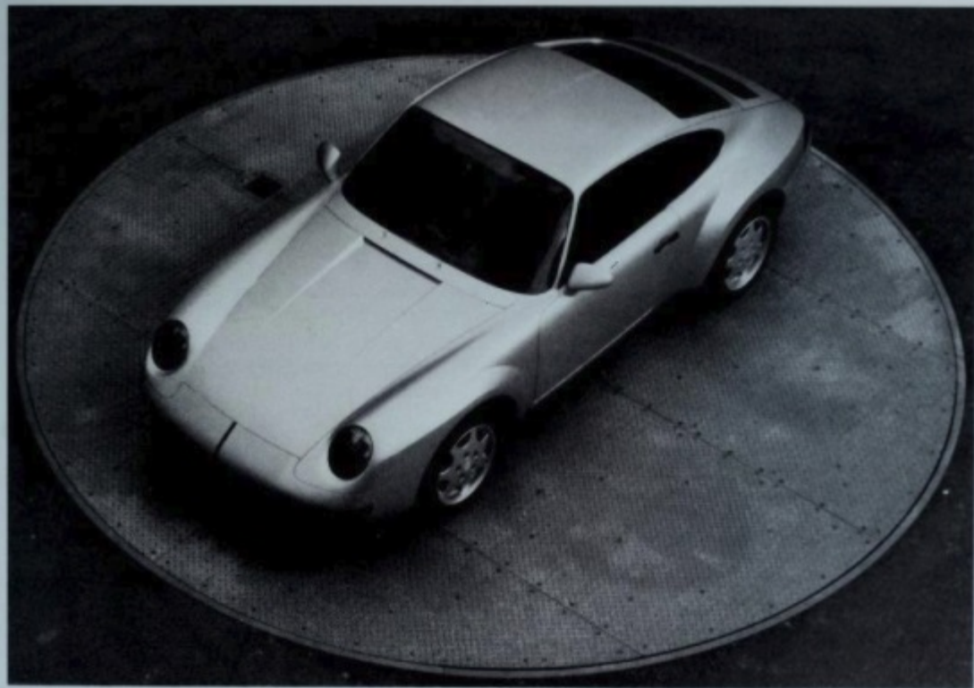
In viewing yard behind the Weissach studio, full-scale models were repeatedly contemplated under natural lighting conditions. The development stage shown here does not yet have fully developed fender contours.
