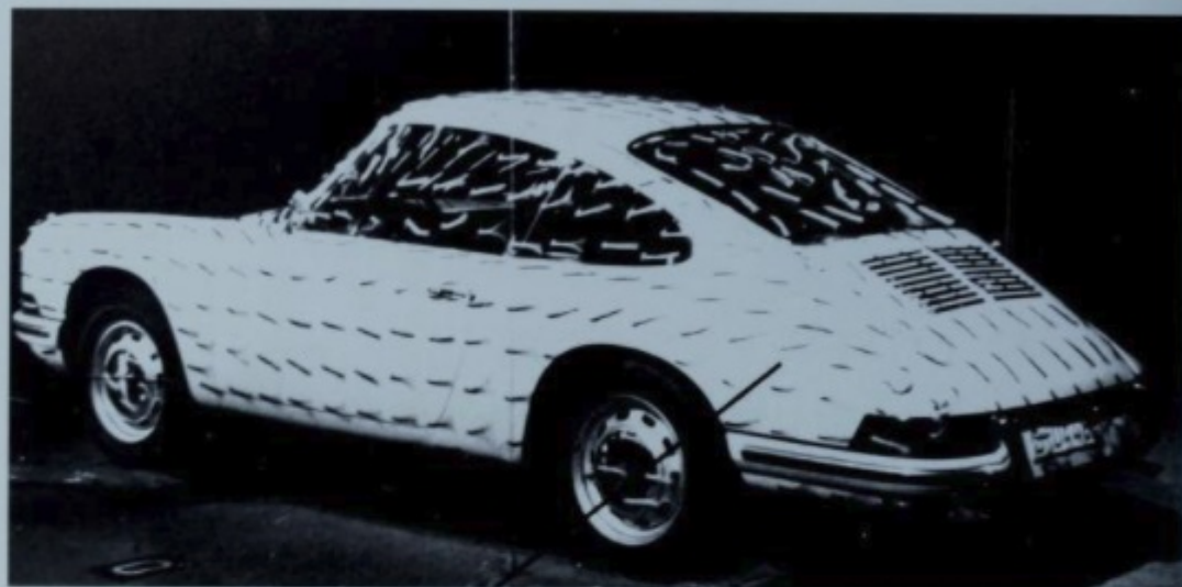
Wind tunnel tests with a full-size model were not carried out until March 1964. The tufts on the backlight indicate far less turbulence than had been noted in the T7 tests. Overall, the results were quite satisfactory.
