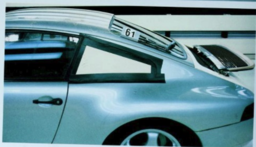
The final stage of Project 993, undergoing wind tunnel testing. Headlights and wheels do not represent production pieces.
