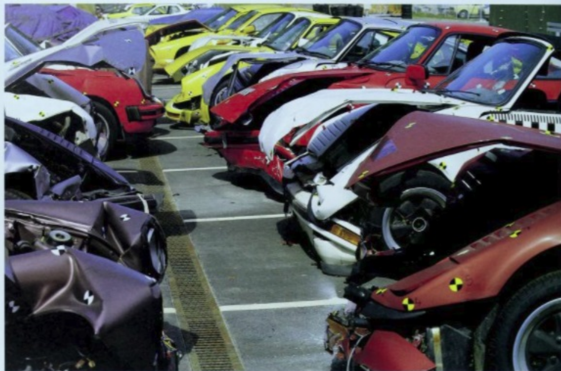
At Weissach, Porsche doesn't skimp on crash tests. After evaluation, the wrecks are scrapped.
