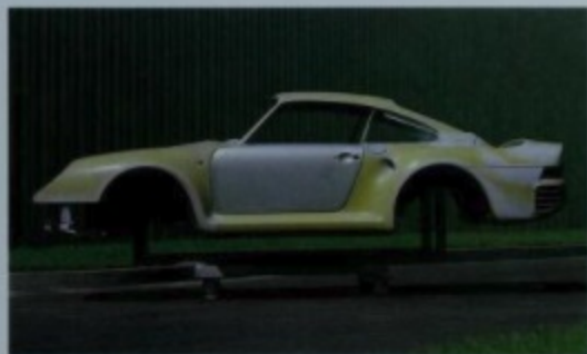
Doors and front lid were of aluminum.
