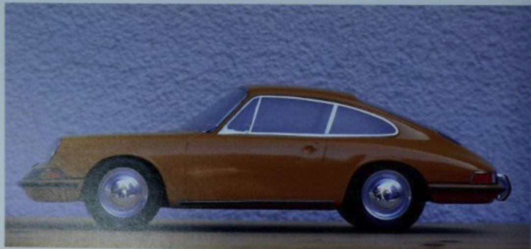
From the end of 1961, development work concentrated in a direction defined by the Type 644 T8. The first model, in 1/12 scale, still envisioned a wheelbase shortened to 2100 mm.
