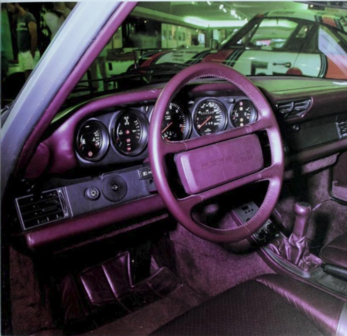
The cockpit of Porsche's technology showcase, the 959, recalls that of the 911. Two knobs on the center console control ride height and shock absorber damping.
