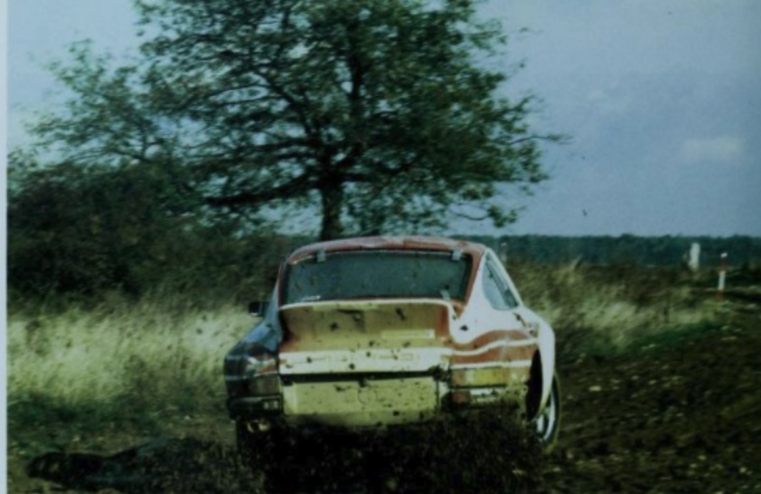
Endurance test: the Carrera RS was also tested for rally applications. For the East African Safari, Porsche installed 210 hp production engines, but modified the suspension.
