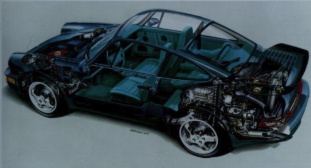
The power and the glory. The 3.3 liter Turbo powerplant needed every inch of available space in the engine bay. The shape of the rear spoiler had to be modified to carry the charge-air intercooler.
