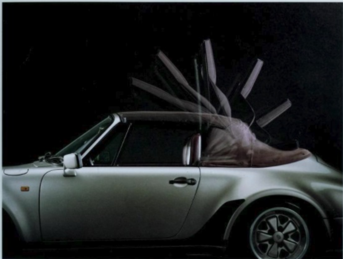
The drive motors for the electric top must actuate 13 movable bows, as well as the roof frame and linkage levers, with 22 pivots.
