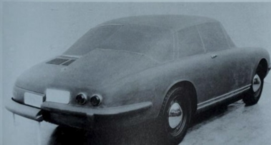
For this design, the Porsche designers adopted the small round taillights of the Goertz proposal.
