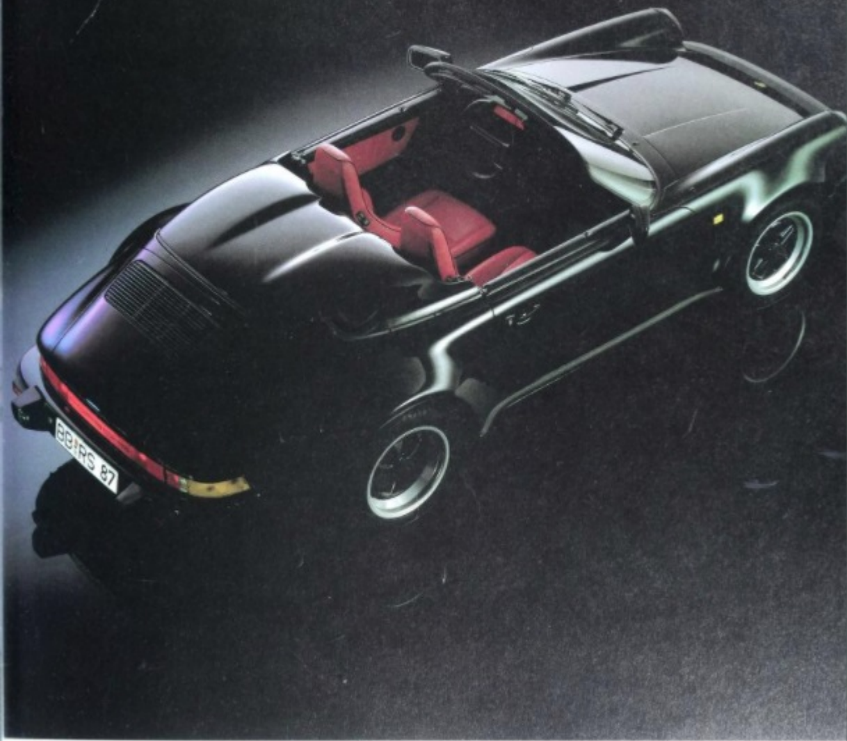
Even before the new worry off, the 1989 Speedster was a classic. The manually operated roof disappeared under the twin fairings of the composite rear deck cover.
