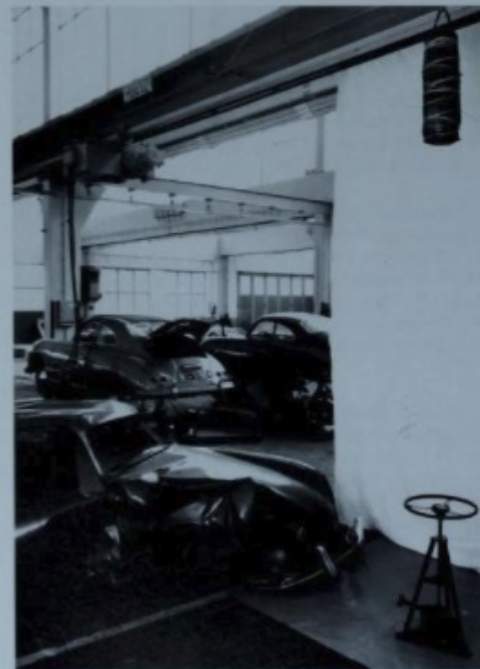
Chief designer Leopold Schmid used sand bags to simulate impact with a steering wheel.
