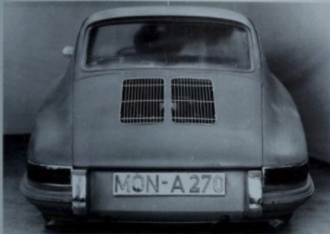
Butzi Porsche created six proposals for the rear air inlet grille. The solution shown at left is that of the 356.
