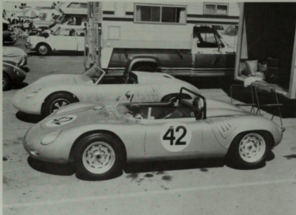
★★★★ The model 718, known as the RSK, was introduced in mid-1957 as the successor to the 550A/1500RS. The RSK utilized the same space frame, and the wheelbase and track were the same as the 1500RS, but the body was thinner, reducing aerodynamic drag somewhat. In 1958, some RSK's had small fins on the rear fenders, and a center-seater was built for Jean Behra to race at Reims as a Formula 2 car. In the top photo the foreground car is a standard RSK while the car behind it is a new "RSK" body built on a 911 chassis by Jack Hagemann. Author photo.
