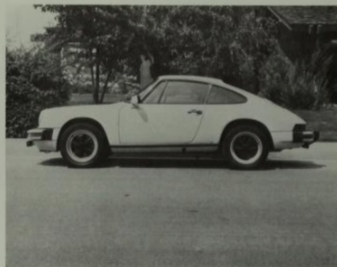
Nineteen years after the 901 was first shown to the public, the basic body shell was unchanged; the wheel openings were flared, the bumpers protruded farther out from the body, and several styles of alloy wheels were available with fatter tires, but the total look was not unlike 1963—which is just fine with me. Author photo.
