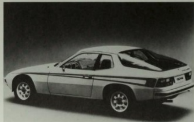
A Championship Edition 924 was offered in February 1977, to commemorate Porsche's winning the 1976 World Championship of Makes. This special edition of 2,000 cars came in one trim: all-white body with red, white and blue side stripes; white alloy wheels; red corduroy seats with blue piping; red carpeting in both passenger and luggage areas; leather-covered steering wheel; and anti-roll bars front and rear. Porsche-Audi photo.
