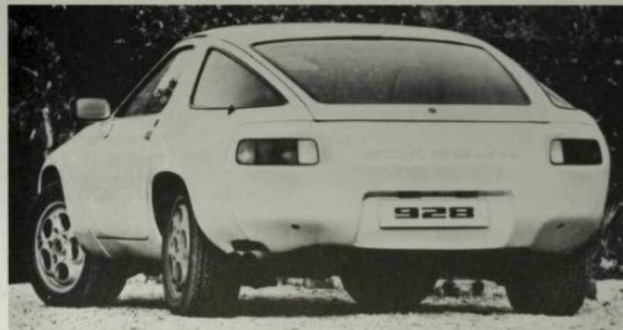
From the rear the American 928 differed from its European counterpart by the addition of running lights and rubber bumper inserts around the license molding. Porsche+Audi photo and Porsche Werkfoto.
