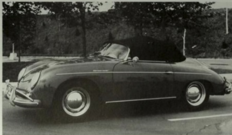
Speedsters, like this early 1957 1600 Super with chromed wheels and hubcaps, looked better with the tops down. Early 1957 models had the "moon" hubcaps, and high bumper uprights that helped protect the delicate Porsche bodies from most of the aggravated assaults by larger cars. All Speedsters had the thin chrome strip along the body side in line with the door handle. Author photo.
