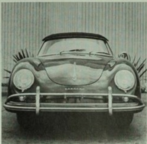
The front bumper "bow" was raised during the 1959 model run to give a bit more protection. The Convertible D, left is an early '59; the Coupe, right, is a late '59. Ralph Poole/Author photos.
