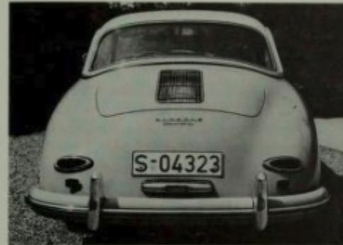
Rear of the 1958 Carrera looked almost like the pushrod Porsches of the same period, but dual exhaust tips were under the bumper instead of through the lower end of the uprights. Porsche Werkfoto.
