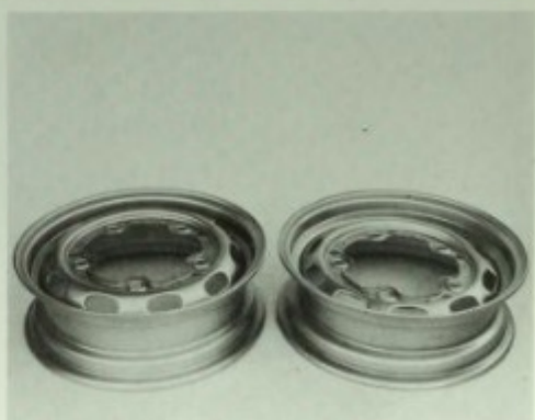
Carrera wheel, left, has steel center and 4 1/2-inch-15 alloy rim, while the 356A is a 4 1/2-15 all-steel wheel. The Carrera wheel has different offset to allow for 20-mm-wider drum. Author photo.
