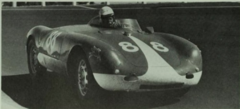
★★★★ When the 550A/1500RS came out, it had smoother front fender/light treatment; sometimes fairings covered the headlights as on Jack McAfee's 88. The factory cars had tubular space frames, the customer 550A still had the tubular ladder-type frame of the 550 Spyder. Ralph Poole photo.
