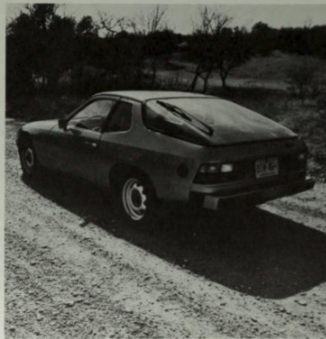
Aerodynamic efficiency and cargo space dictated the shape of the rear, but it was one of the least appealing views of the 924. The rear window wiper was part of the Touring Package II for the U.S. market in 1977. The rear window/hatchback lifted for luggage stowage and access. Porsche+Audi photo.
