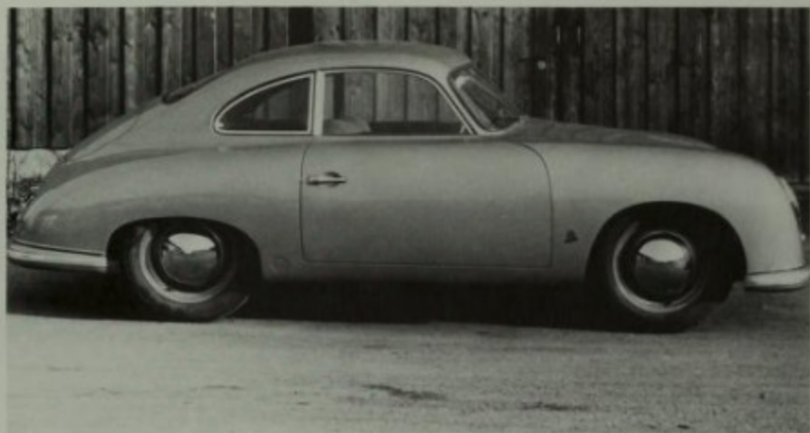
In 1950, production started in Stuttgart and the cars acquired windshields with the ends rounded for better airflow to the body sides. The bodies were made by Reutter (note the unusual Reutter emblem on the side). Kurt Werner/Road & Track photo.
