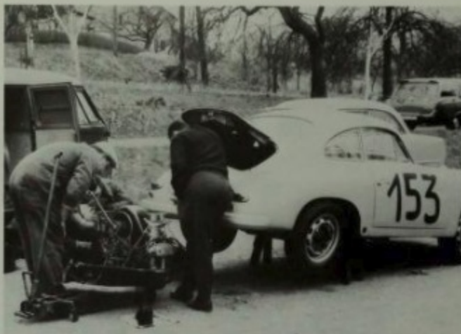
It was often easier to remove the Carrera engine than it was to work on it in the car. This was a private entry at the Eberbach hill-climb in 1962. Kurt Worner/ Road & Track photo.
