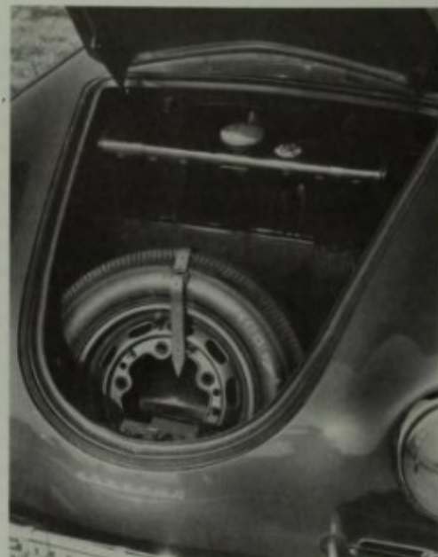
Even with the spare tire mounted more vertically in the front, the huge square gas tank kept the useable space to a minimum. Most Porsche travelers utilized the space behind the front seats for larger luggage pieces, putting things they wanted to hide in the front. Ralph Poole photo.
