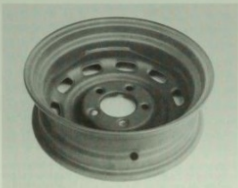
The 4 1/2-inch wheel for the 356C was all steel and welded together as with other Porsche steel wheels. The bolt circle was smaller than before due to the hubs used with the new disc brakes on the C models. Author photo.
