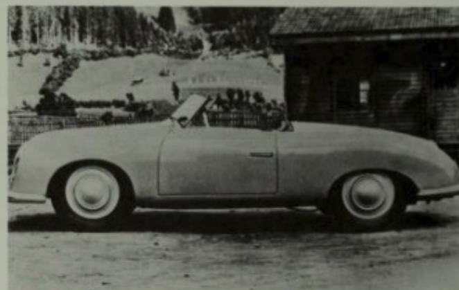
The first Porsche, as it looked when completed in Gmünd, Austria, in May 1948. It was a mid-engined car with an aluminum body designed by Erwin Komenda.
