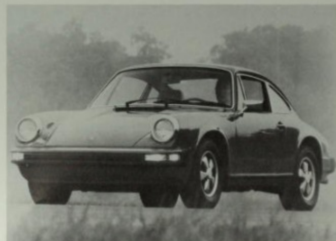
The 912 was revived in 1976 after the 914 was dropped, and looked even more like the 911. The new 912E had the four-cylinder, fuel-injected engine from the VW 411 and was rated at 32 highway mpg by the EPA. Porsche+Audi photo.
