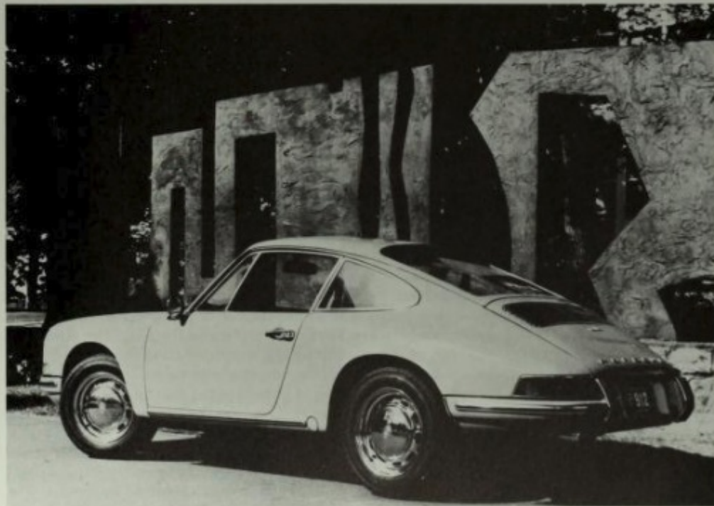
The 912 (this is a 1969) was so much like the 911 in appearance that only very knowledgeable observers could spot the difference without looking inside to see the less-fancy interior or into the engine compartment. The rear lid carried a 912 just below the air intake grille. Porsche+Audi photo.
