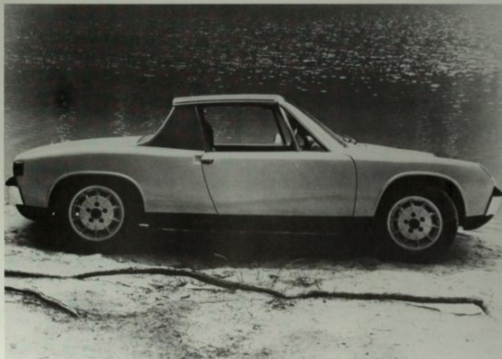
The 914/6 could be identified by five-lug wheels. Shown here are Mahle die-cast magnesium wheels which were optional. Porsche-Audi photo.
