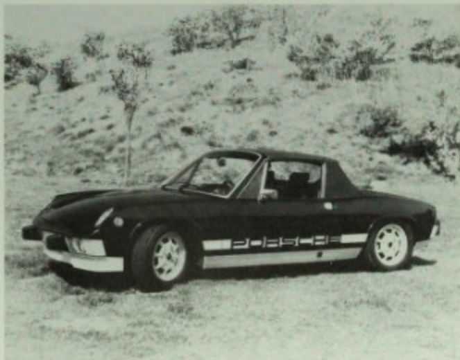
Introduced in April 1974 was a limited-edition 914 which had a front spoiler, alloy wheels, a special interior and only black or white body colors with contrasting accent trim. Porsche+Audi photo.
