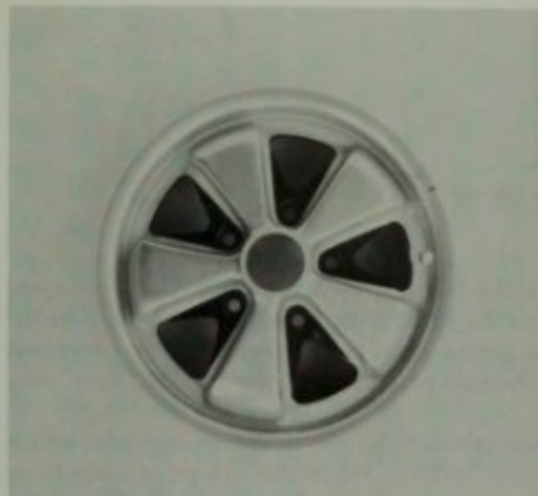
The 1967 911S 4J-15 one-piece, forged-alloy wheel, by Fuchs, has now become popular on any model Porsche that has the right bolt circle. Author photo.
