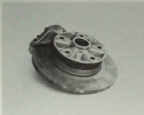
Disc brake and caliper for the 356C were made by Ate under license from Dunlop. The rear disc incorporated a small drum-type parking brake which was operated mechanically. Author photo.
