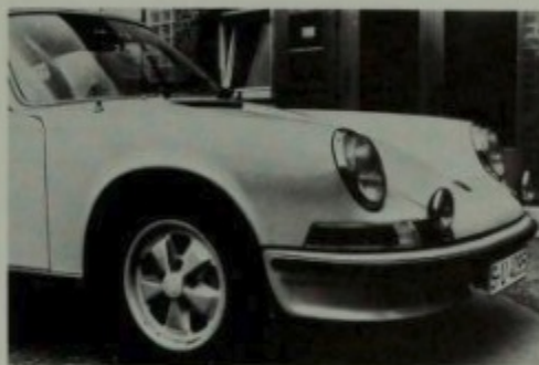
The 911S for 1972 came equipped with a front "air dam" or "spoiler" which reduced front end lift from 183 to 102 pounds at 140 mph--the top speed of the S. The spoiler was optional on the T and E, and became so popular that it was made standard equipment on all three models later in 1972. Porsche+Audi photo.
