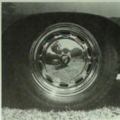
A flat hubcap with the Porsche crest signified a disc-braked 356C. Author photo.
