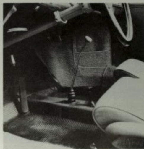
This early 1957 Speedster has the heater control behind the shift lever, which was standard for that time. In mid-model run positions were switched—shift lever behind the heater control. Author photo.
