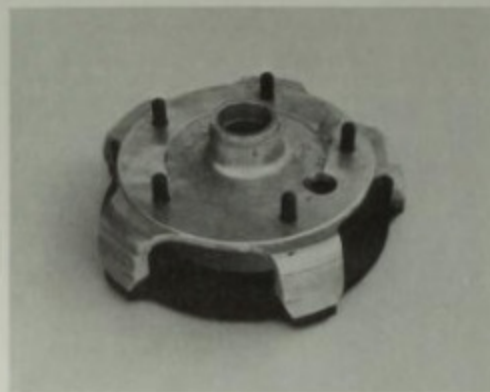
Porsche's own disc brake design, sometimes referred to as a "ring disc" brake, had the caliper on the inside, with the disc and hub attached at their peripheries in order to utilize the wide bolt pattern of the early Porsche wheels. In spite of this brake's light weight, Porsche would have been the only car company using it so the limited production would have made the unit cost extremely high. Author photo.
