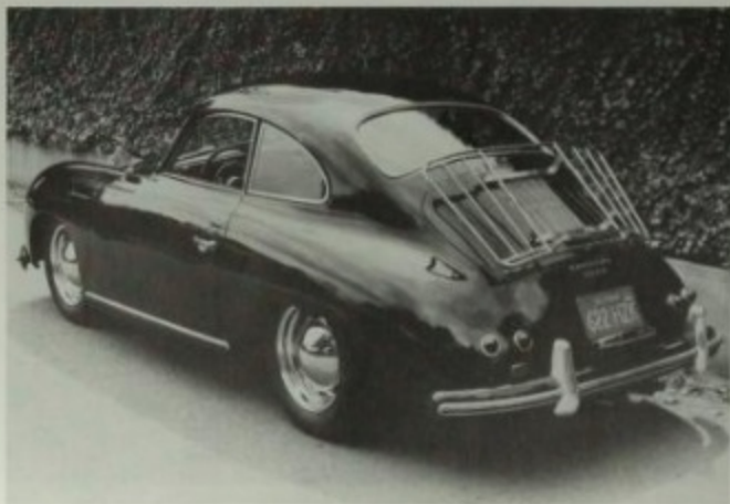
Extras—factory or aftermarket—have always been popular with Porsche owners. This 1955 Continental has a luggage rack attached to the air intake grille (no self-respecting Porsche owner would drill holes in the body to attach one), chrome wheels and an Abarth exhaust system. Ralph Poole photo.
