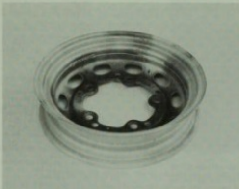
The 3 1/4-inch-wide wheels of the 356 had the rim and wheel center welded together and carried the large-diameter bolt circle to match the Volkswagen brake drums used on the early cars. Author photo.
