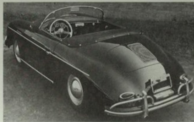
The side view of the 1958 Speedster is almost identical to the 1957, but this one has the louvered trim rings around the hubcaps. The dash looks much like the 1956, and '57; but this one has a radio installed in front of the passenger and the steering wheel is from an older model. The rear looks much like a late 1957, with the low license-plate light, teardrop taillights and two-piece upper bumper bar; but the exhaust through the lower part of the bumper uprights indicates it is a 1958. Ralph Poole photo.
