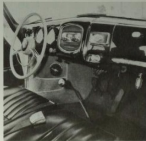
A 1955 356 Continental Coupe interior. Fuel reserve handle and fuel filter were under dash. The radio is an aftermarket unit made by Motorola. Author photo.
