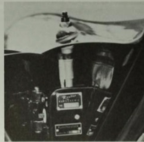
The serial number (107819) on the Reutter Karosserie plate identifies the car as a 1959 356A/1600 Coupe with a Type 616/1, three-piece crankcase engine with two 32 NDIX Solex carburetors. The engine bore and stroke are 82.5x74 and with a 7.5:1 compression ratio the engine delivers 60 DIN hp at 4500 rpm. Author photo.
