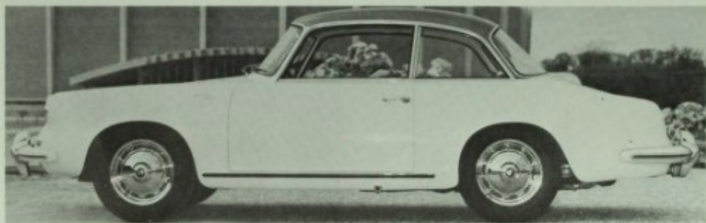
*** Karosserie Beutler, in Thun, Switzerland, produced several bodies for Porsche running gear. This is a four-passenger coupe based on the 1962 356B. Bumpers, lights, door handles, wheels and hubcaps appear to be stock items. The wheelbase also appears to be unchanged from the stock 82.7 inches. Road & Track photos.
