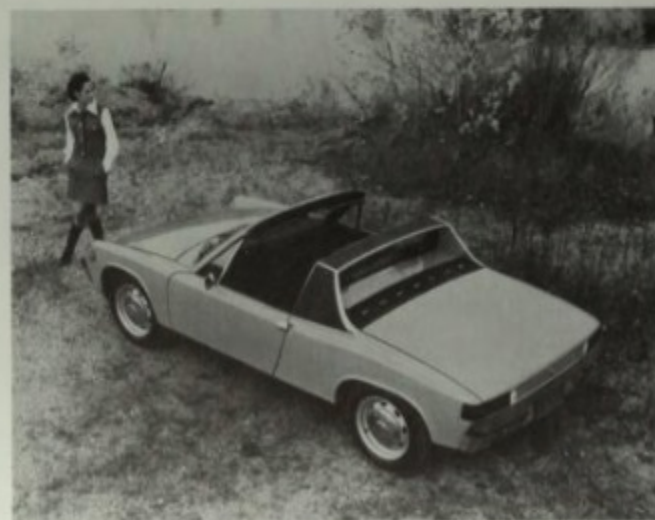
All 914's had the removable roof section and fixed Targa-type roll-over bar. The only Porsche identifying feature on the outside was the lettering on the engine air intake behind the roll bar. This is a 1971 model. Porsche+Audi photo.
