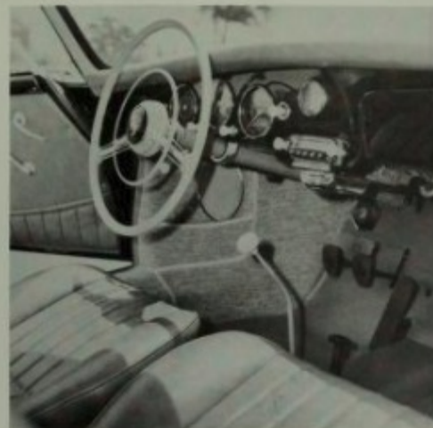
Interior of the 1959 356A 1600. A clock has been added to the center of the dash above the radio, the fuel reserve switch can be seen just under the dash at right, the radio speakers mounted in the carpeted kick panels. The windshield washer was activated by the left foot (above brake and clutch pedals). Author photo.
