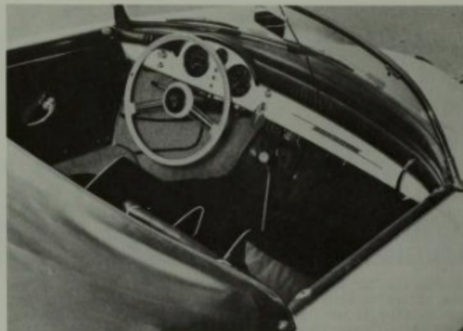
The 1955 Speedster interior displayed the functionally stark design. The Cabriolet and Coupe still had the "bent in the center" flat vee windshield with curved outer edges but the Speedster had a fully curved windshield—a style that would be adopted by all Porsche models late in the year when the 356A was announced. Ralph Poole photo.
