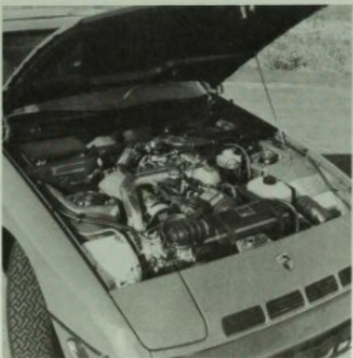
The 924 Turbo engine with its KKK (Kuhnle, Kopp & Kausch) turbocharger produced the sort of performance the 924 should have had in the first place for the U.S. market. Author photo.
