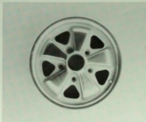
The 911E used this 5J-14 single-piece, forged-alloy wheel as oem equipment. Aside from appearance, the main advantage of an alloy wheel is light weight and more precise tolerances (lateral and vertical runout—concentricity between hub and rim). Author photo.
