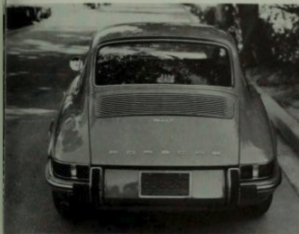
The 911 C series was introduced in September 1969 as 1970 models, and had engines that displaced 2195 cc. These cars carried a decal of an engine silhouette with 2.2 superimposed on it in the back window of each car, as on this 1970 911T coupe. Porsche+Audi photo.
