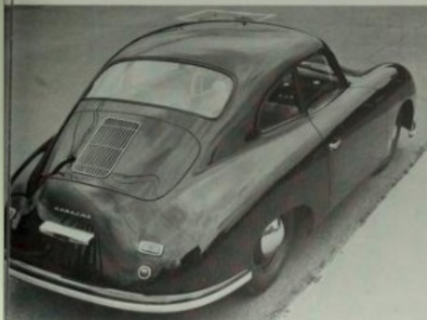
Stuttgart-built coupe of 1950 had the form that would continue through the 1955 model year; steel body by Reutter, with two-piece windshield (flat in the center and curved at the outer edges), two round and two rectangular lights flanking the light bar over the rear plate and a single round parking/turn-signal lens under each headlight. The Porsche lettering was now standardized in design and mounted front and rear under the opening lids. Author photos.
