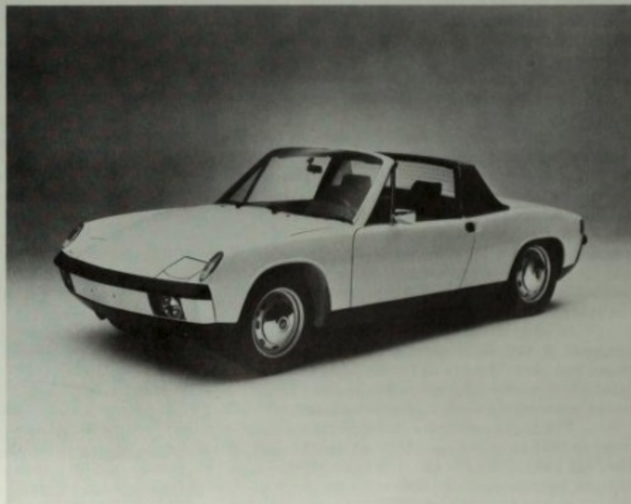
Standard 914 for U.S. had side-marker lights just behind front turn indicator lights, and the European version had driving lights set into bumper face-bar. Porsche+Audi photos.
