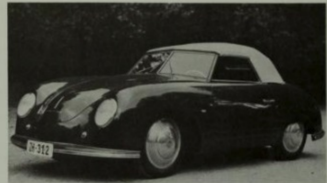
Beutler, in Switzerland, built six of the eight Cabriolet bodies for the Gmünd 356/2 series cars. They had two-piece flat-glass vee windshields and full-wheel discs. The Porsche lettering was on the front lid, unlike later models which had it below the opening.
