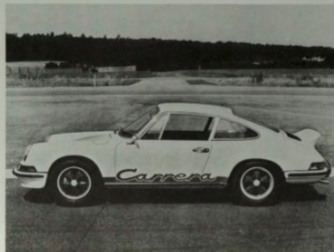
The Carrera name returned to the Porsche line in 1973 on the 911RS (for Rennsport, or race sport). It had a 2687 cc engine, no sound insulation, thinner sheet metal and glass, fiberglass rear lid with a small ducktail spoiler, and no emission equipment so it couldn't be sold for road use in the U.S. (it was raced in the U.S. however). It was popular as a road car in Europe. Porsche+Audi photo.
