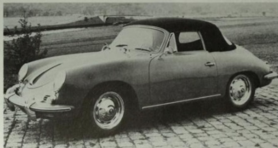
The 356B, in 1960 and '61, had the T-5 body with the high bumpers, raised-center hubcaps and headlights mounted higher on the front fenders which made the fender line straighter from the windshield to the top of the light (when compared to the 356A). The front compartment opening was rounded at the leading edge. Shown is a standard Cabriolet. Porsche+Audi photo.
