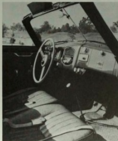
A 1955 356 Cabriolet with similar dash to the Continental, but different detailing. This radio is a Telefunken. A special floor mat has been fitted over the stock rubber mat.
