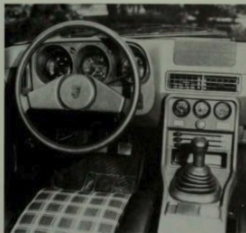
Steering wheel rim of the 924 was not concentric with hub (offset toward the top), for better instrument visibility and more leg room. It was still a tight fit, and got worse as the wheel turned.
