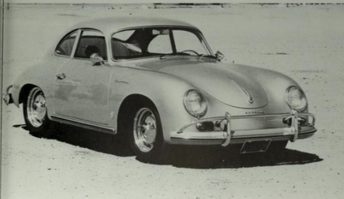
A Carrera 356A Coupe, which the high front bumper "bow" identifies as a late 1959 unless the owner has added it later. The rear view mirrors are after-market items. The deluxe hubcaps were standard on the Carrera GS, but were often added to other models by owners.
