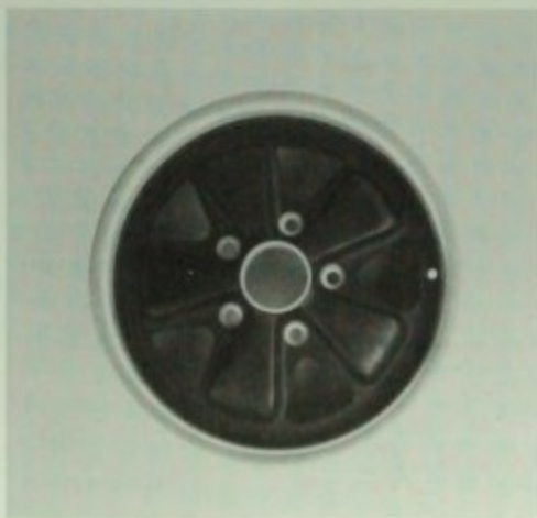
The late 911 6J-15 alloy oem wheel was similar to the early wheel, but with blacked-out spokes. It was also a forged wheel. Author photo.
