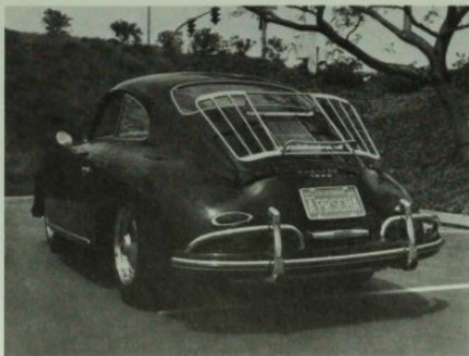
A 1959 356A 1600 Coupe with all the extras, including an accessory luggage rack for the rear deck. The grille on the engine lid is for air intake, so the luggage doesn't get as much heat as one might expect from this location, but it does add weight in the wrong place: high and behind the rear axle. Author photo.
