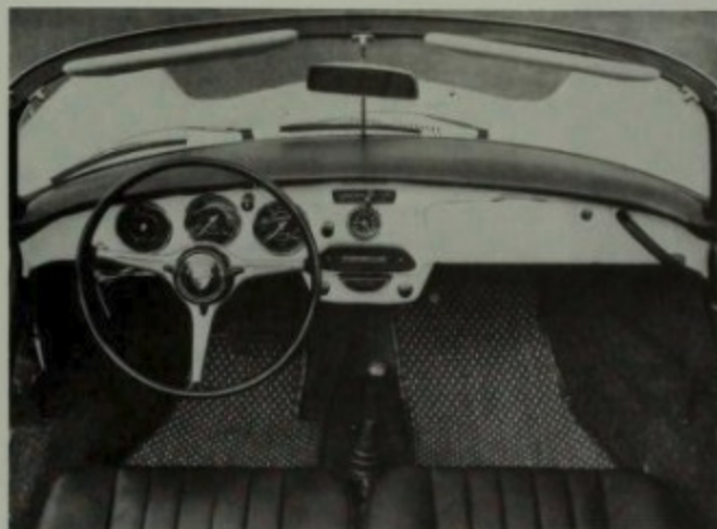
This dash shot of an early 356C—a 1964 built in 1963—shows the glovebox, grab handle and padded sun visors available on the C series. On the 1964 models the handgrip was eliminated and the light switch moved from behind the steering wheel where it was easier to reach. Porsche Werkfoto.
