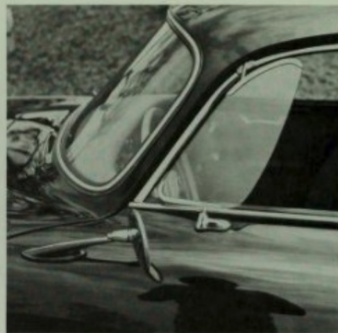
The 1959 Coupes, this one a 356A 1600, didn't have vent wings built into the door, but had a factory option pivoting wind wing on the outside. Author photo.
