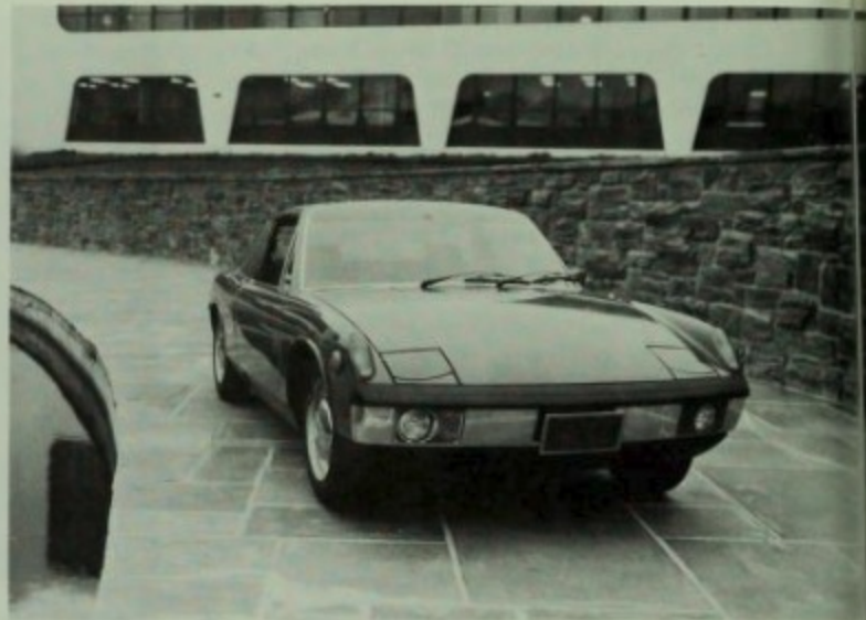
The U.S. version of the 914 received the European-style bumper-mounted driving lights in 1972. Also new were improved ventilation and an adjustable passenger seat as standard, but no other visual changes. Porsche+Audi photo.
