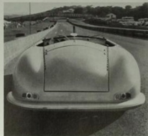
Porsche number 1; the matriarch—or patriarch, depending on your perspective—of all Porsches. The aluminum body covered a Volkswagen suspension and modified VW engine, held together by a space frame. Unlike future road-going Porsches, the engine was ahead of the rear axle. It has been recently restored (but not to original specs) by the factory. Author photos.
