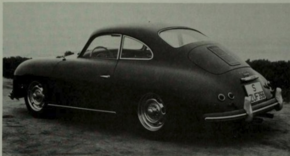
A 1956 Porsche 356A 1600 Super, equipped for German delivery. The chrome-plated wheels and center-lock hubs were optional equipment. The hub nuts had no “wings” or “ears” because of German restrictions on projections that could harm pedestrians. Projecting radiator ornaments (which wouldn’t affect Porsche) were outlawed at the same time. Author photo.
