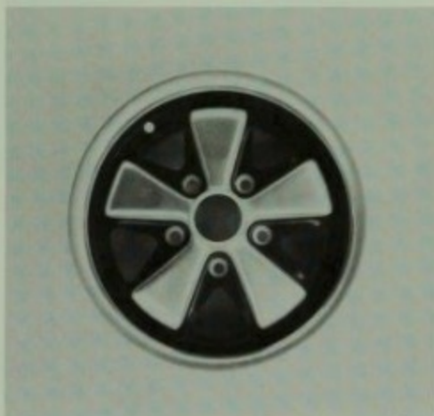
An early 911 6J-15 oem wheel. Most factory-installed alloy wheels are forged (some are pressure cast), but some aftermarket suppliers offer cast-alloy wheels in similar patterns. Author photo.
