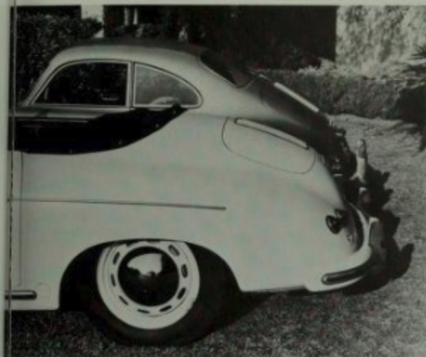
The Coupe style lent itself to a rear-engined design because it easily covered the vertical fan, but the Speedster and Cabriolet required more "hump" in the back than might otherwise be used for a notchback design. Ralph Poole photo.
