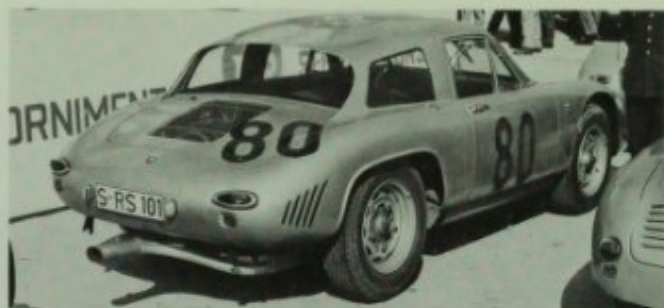
***** Herbert Linge and Edgar Barth shared the wheel of this 2000 GS GT to finish third overall in the 1963 Targa Florio. It was on a 356B chassis with Carrera 2 engine. Only two were built. Author photo.
