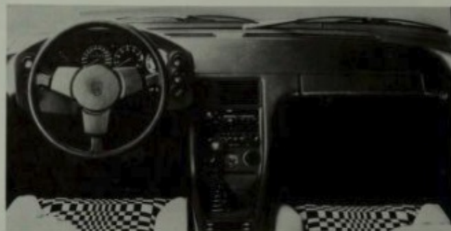
The steering wheel of the 928 didn't adjust in and out, but moved up and down—with the instrument cluster—to keep it in view of the driver at all times. The glovebox was air conditioned along with the interior. Porsche+Audi photo.
