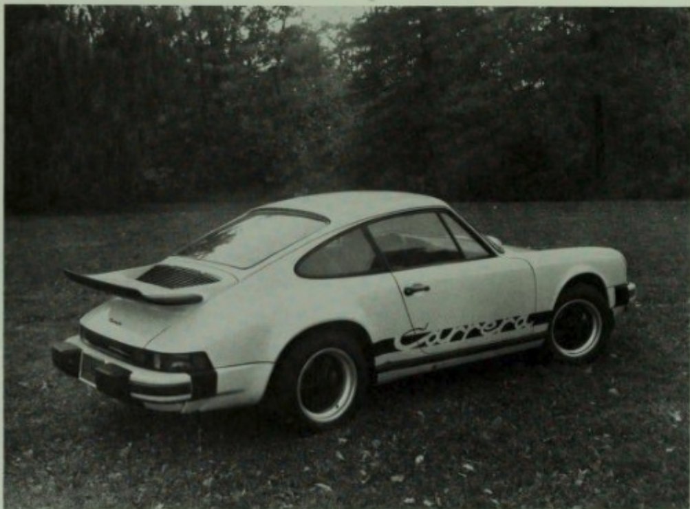
In 1975, the Carrera got what is now referred to as the "whale-tail" rear spoiler. This device was designed by Porsche for the 930 Turbo and 935 race cars so it had plenty of development before application to the Carrera. Porsche+Audi photo.
