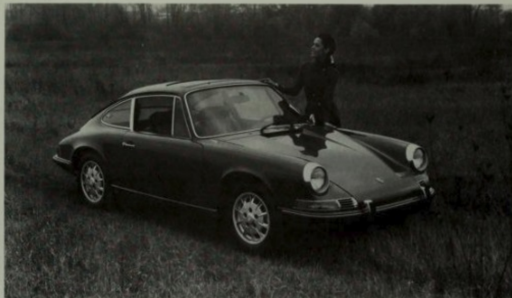
In 1971, the 911 was still available with either Coupe or Targa body, four- or five-speed all-synchromesh or three-speed Sportomatic transmissions, and with T, E or S engine tune. This is the T, with optional sunroof and ten-spoke alloy wheels. Porsche+Audi photo.
