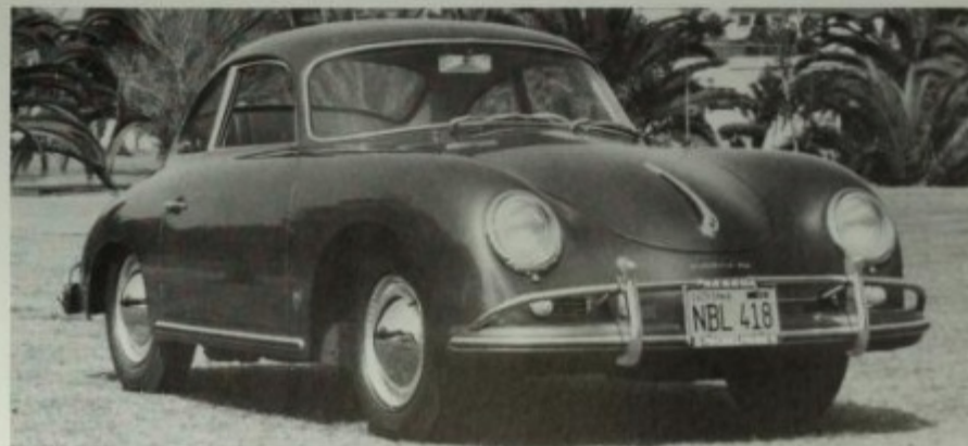
This 356A 1600 shows the way most Porsches were equipped for American delivery in early 1957: with vented wheel rings (around the plain chrome hubcap) and one-piece front bumper "bow" connected to the tall uprights. Ralph Poole photo.
