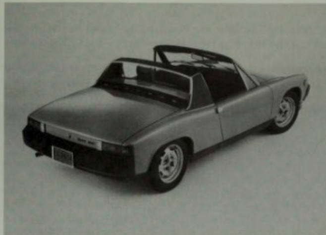
For 1975, the 914 received new energy-absorbing impact safety bumpers which had 2.5 inches of "give" via hydro-pneumatic dampers and new wheels; but the basic body remained as before. Porsche+Audi photo.
