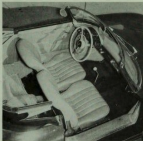
The 1959 Convertible D, with body by Drauz, was a continuation of the Speedster but with roll-up windows, higher top, coupe seats and more luxurious trim. Ralph Poole photo.
