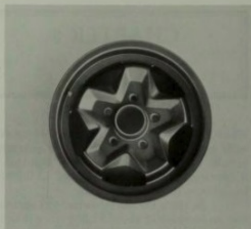
"Cookie cutter" alloy wheel by ATS comes in 15x6- or 7-inch rim widths. This wheel has also become popular on a variety of Porsches. Author photo.
