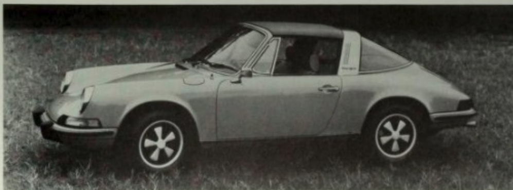
The 1973 911T Targa with the top on showed how open-air motoring could be done in relative safety, as the Targa "T-handle" was also a roll-over bar. Options included choice of three engines, three transmissions and forged-alloy wheels. The bumpers were made stronger for 1973. Porsche+Audi photo.
