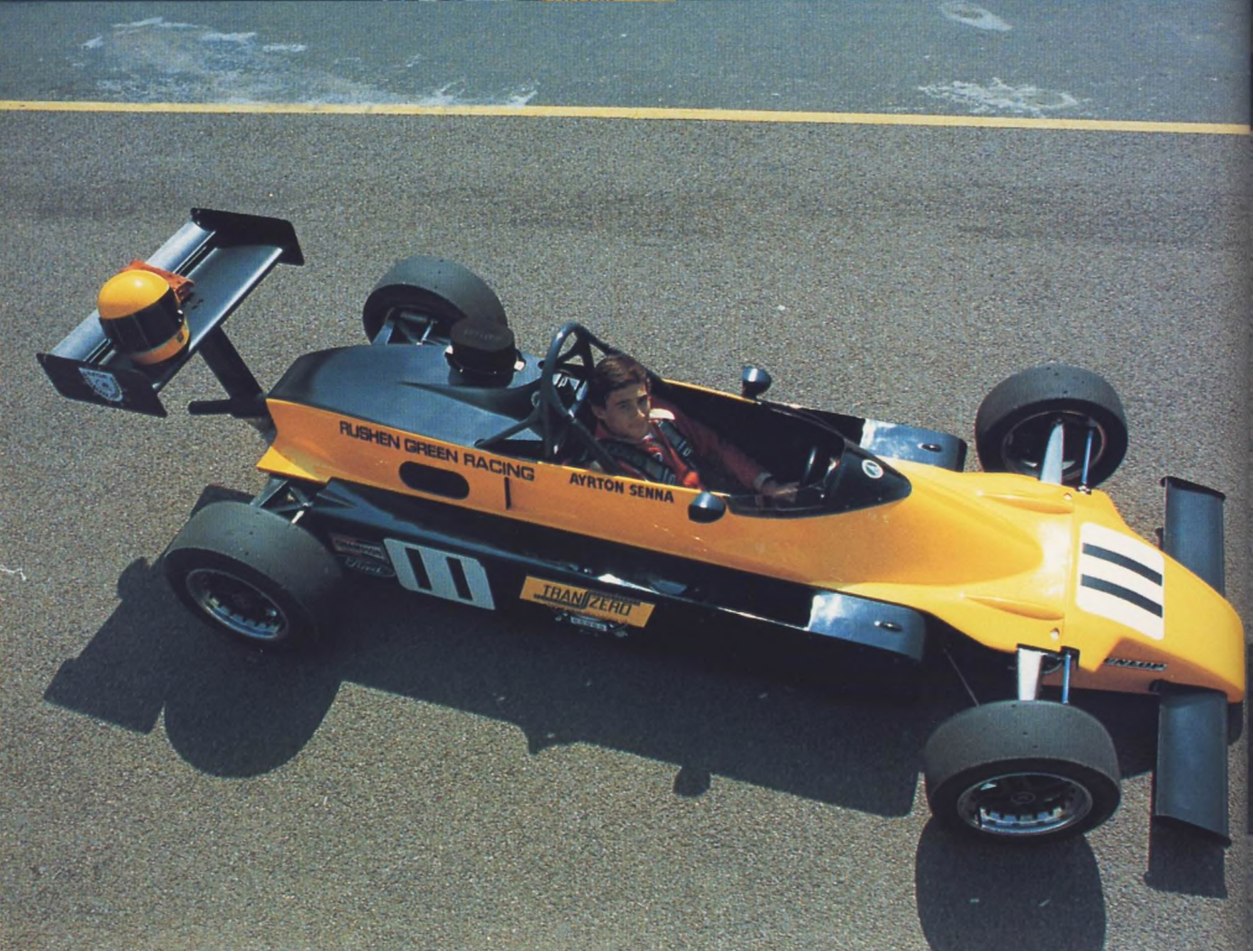
Van Diemen's excellent FF2000, basically a regular FF1600 car using wings and slick tyres, was used for the British and European championships – and won both
