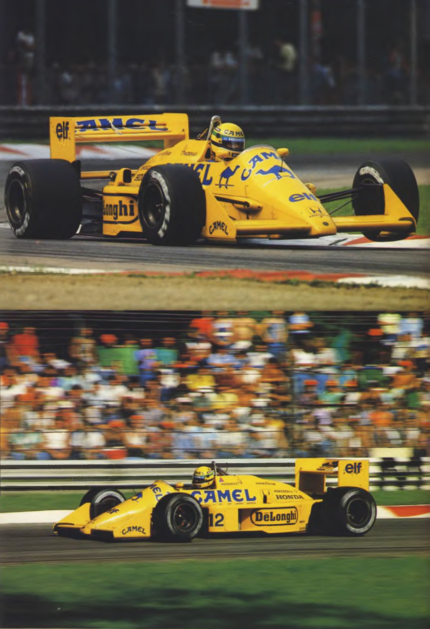
Though the 'active' Lotus-Honda was effective on slower street-type circuits, it suffered on high-speed tracks. Not even a switch to 'lo-line' bodywork inspired by the Williams improved the situation
