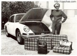
In view of considerations given to body dimensions, it became necessary to consolidate the new components into a compact unit. The inside space has been enlarged while keeping the outside dimensions down—here exceeding the overall length of the Type 356 by only 120 mm, yet reducing the overall width by 70 mm. At the same time larger window areas have been provided, to satisfy the demands of today.
