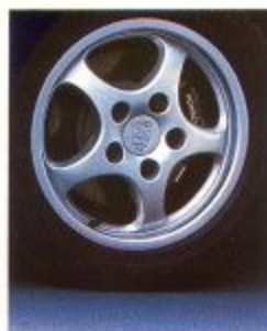
Standard with the Carrera 4: new Cup design wheel, with greater brake cooling capacity.
