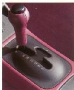
In manual mode, tip the selector forward to shift up, tip back to shift down.
