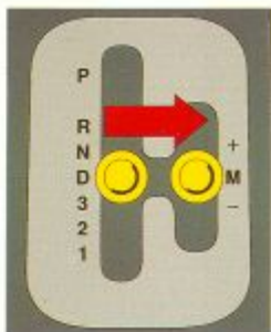
Five shift patterns in Automatic. tip up and back in Manual; computer-monitored in both.
