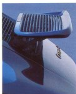
To reduce drag and lift, the extendible rear spoiler engages automatically at about 40 mph.
