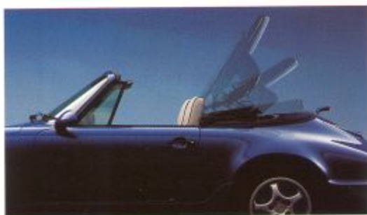
The 911 Cabriolet offers fully automatic top up/down operation: push one button, and motors do it all – even latching and unlatching the locking clips!
