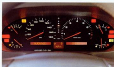
The Driver Information System monitors and prioritizes 22 functions; a flip of the column stalk activates a connected 10-function onboard computer.
