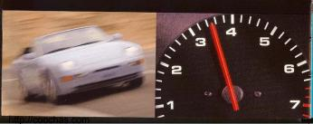
Above 1,500 rpm, the intake valve timing automatically retards to produce maximum midrange torque – peak torque is 225 lb-ft at just 4,100 rpm, far below redline. And above 5,500 rpm, the timing is again advanced for optimum efficiency power.
