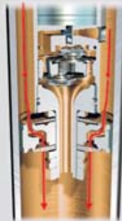
Left: Rebound in 'Normal' mode – damper piston and bypass valve
