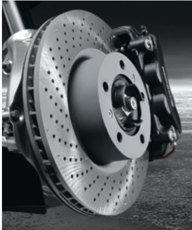
Standard brake system on 911 Carrera 4/911 Targa 4
