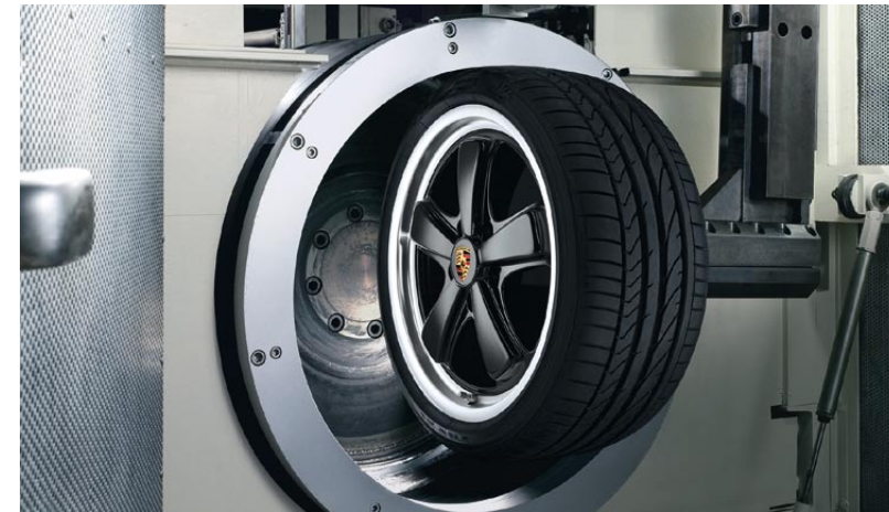
19-inch Sport Classic wheel in the Zwart test (two-axis test rig)
