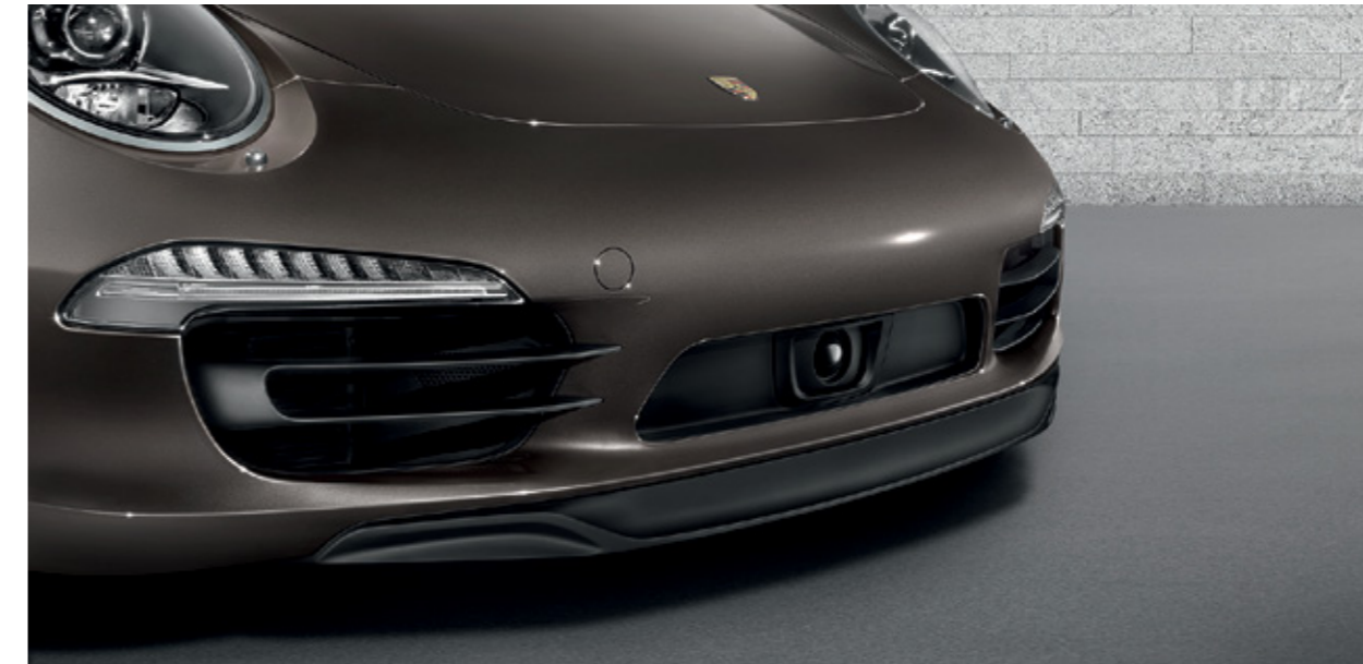
Radar sensor of adaptive cruise control
