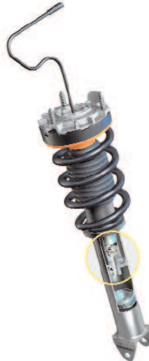
Compression in Normal mode— damper piston with bypass valve open
