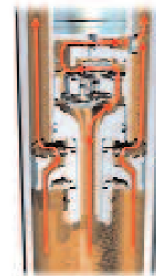
Compression in Normal mode— damper piston with bypass valve open
