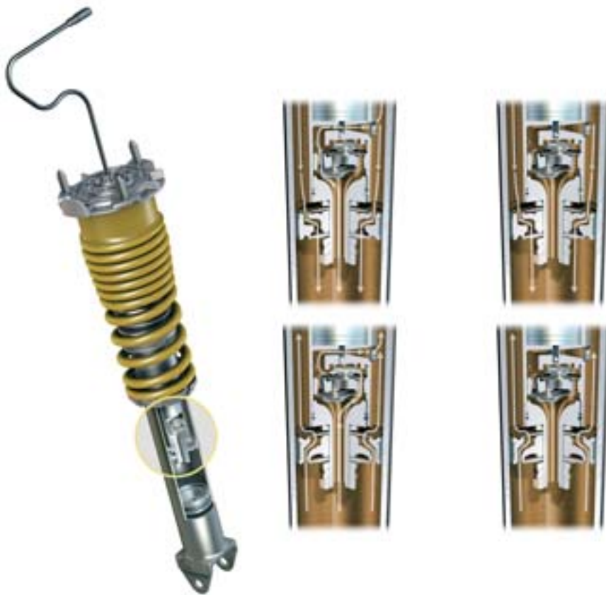
Fig. 19: PASM damper, operating diagram
