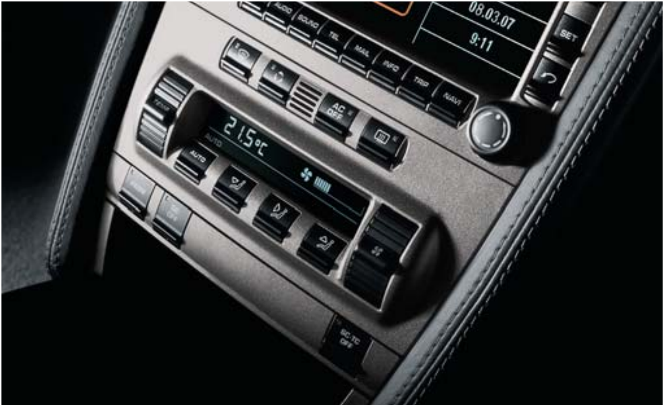
Fig. 21: SC OFF and SC+TC OFF buttons in the control panel/centre console
