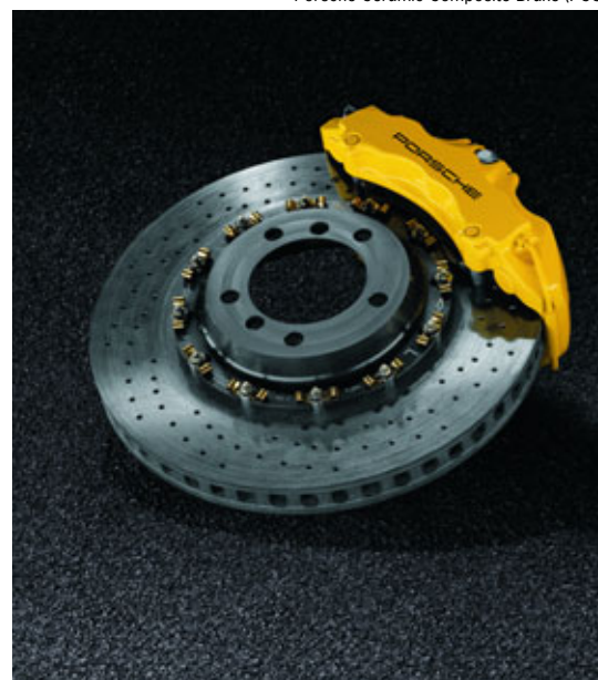
Porsche Ceramic Composite Brake (PCCB)
