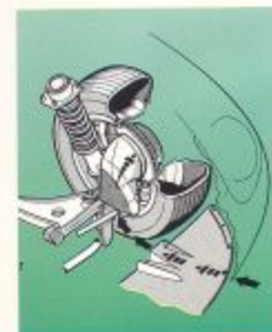
Cooler brakes for safety: air is directed to cool brakes via race-bred air management technology.
