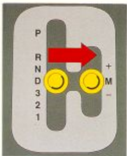
Ingenuous simplicity of Tiptronic in "manual:" tip forward to upshift, back to downshift.
