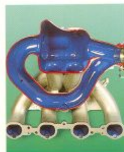
Resonant induction is one of 968 engine's many "torque enhancement" technologies.
