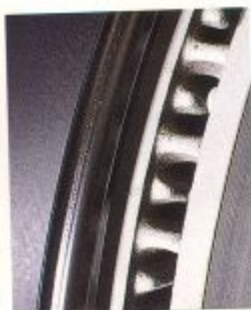
Each 968 disc brake is internally vented for optimal cooling.
