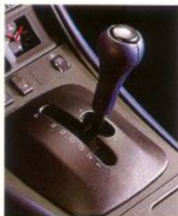
Moving shifter into right gate activates Tiptronic's "manual" function.
