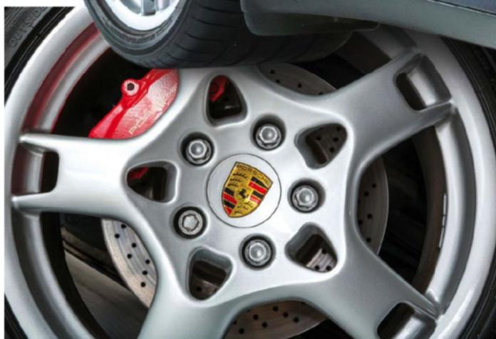
Stylish Carrera alloys cover the 330mm drilled brake discs
