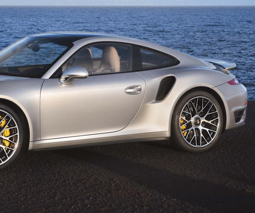
The new 991 platform means the Turbo now has a wheelbase that is 100mm longer than before. Porsche says it weighs just under 1,600kg, or just 25kg up on the 997. For a car with such a wheelbase stretch, that's remarkable: with the extra power and the car's better ability to use it, there's an all-round improvement in performance.
