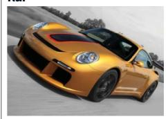
Alois Ruf's 997 Turbo base package takes the 500bhp of the Turbo and 530bhp of the Turbo S to a claimed 620-650bhp respectively – with a remapped ECU following fitment of air filters, sports cats and a larger bore exhaust system. The conversion claimed 656lb ft of torque and 0-62mph in 2.9 seconds, with 0-124mph in 9.1 seconds and 202mph. It was available for both manual and Tiptronic/PDK transmissions.
