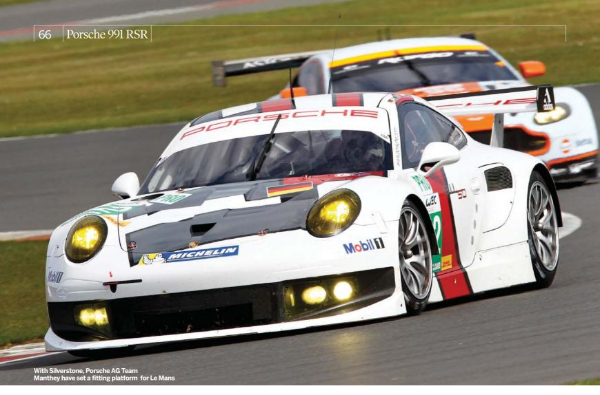
aero package giving less downforce with greater efficiency has been homologated. "We're not allowed to change the rear wing, so we mainly change the front and rear diffusers because these elements create downforce," explains Kristen.
