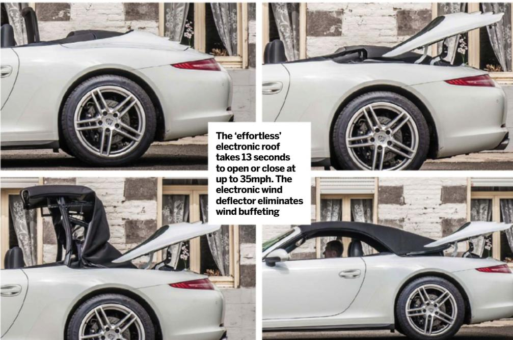
The 'effortless' electronic roof takes 13 seconds to open or close at up to 35mph. The electronic wind deflector eliminates wind buffeting
