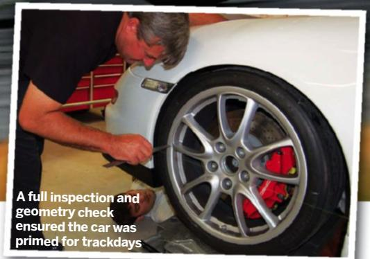
A full inspection and geometry check ensured the car was primed for trackdays
