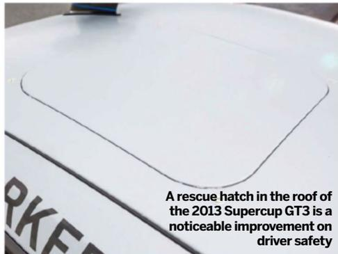
A rescue hatch in the roof of the 2013 Supercup GT3 is a noticeable improvement on driver safety
