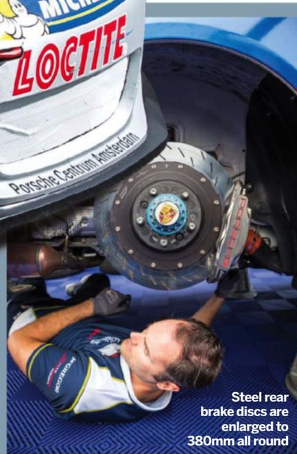
Steel rear brake discs are enlarged to 380mm all round
