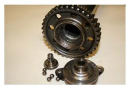
After: Hartech can both fix and prevent IMS failure by using a stronger spindle and replacing the bearing
