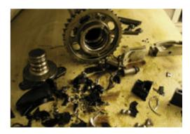
Before: Typical IMS failure results in loose debris circulating through the engine
