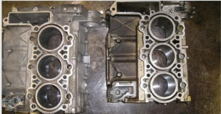
A dissection of the cylinder head (left picture) shows the weak areas susceptible to cracking (top left). This is largely due to manufacturing, highlighted (right picture) by the block casting from a Boxster S on the right hand side, while the left shows the same casting bored out for the Type 996 911, resulting in thinner and weaker cylinder walls
