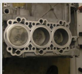
Hartech deal with the problem by boring out a cracked or seized liner (left) and installing a new cylinder (middle). Restraining rings can also be fitted in the top (right) to stabilise the Lokasil bores when re-rounding has been carried out
