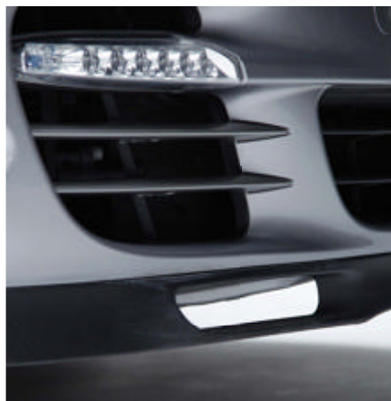
The front spoiler aids aerodynamics and feeds air to the brakes
