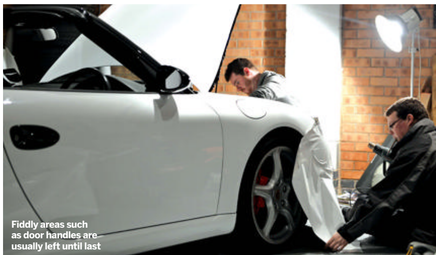
The process is time-consuming, requiring a heat gun to help stretch the vinyl over and round all necessary edges
