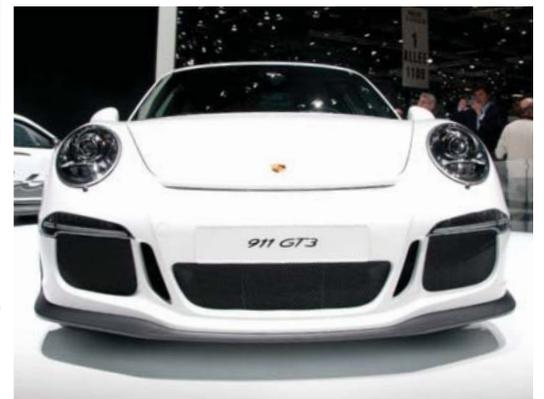
Following the cues of the previous Type 997 GT3, the 991 GT3 has huge, air-grabbing vents up front, a deep front spoiler and the now customary bonnet edge air vents. Vents behind the arches aid brake cooling, while the twin central exhausts separate the GT3 from the standard 991. Sitting 44mm wider at rear, the 991 GT3 nails that typically hunkered down stance. 20-inch centre-lock wheels shield 380mm carbon ceramic disks and six-piston calipers, assuring the GT3 of big stopping power
