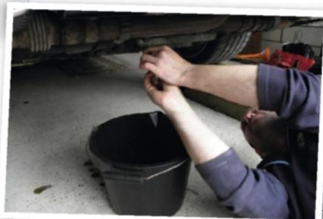
One of the first steps was draining the coolant fluid from the M97s system
