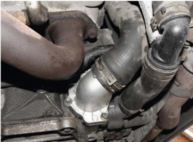
was caught in another bucket. The adjoining part to the thermostat was cleaned down using wet/dry paper. Using some Loctite 5922 glue, the new gasket was sealed onto the new thermostat. Luckily, fitting it back onto the engine wasn't as much hassle as taking it off, but you will still need those specialist sprockets.
