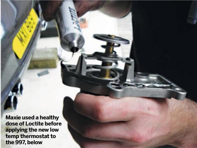
Maxie used a healthy dose of Loctite before applying the new low temp thermostat to the 997, below
