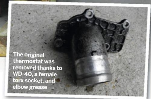
The original thermostat was removed thanks to WD-40, a female torx socket, and elbow grease
