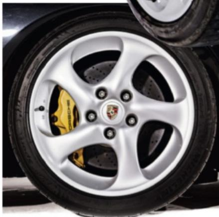
18-inch Turbo-style alloys hid expensive PCCB brakes. GT2s from '04 got lighter ten-spoke wheels
