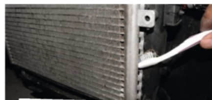
Removing the front bumper gives better access to home the third radiator. This also presents a good chance to remove any road debris from the other front radiators before reassembly
