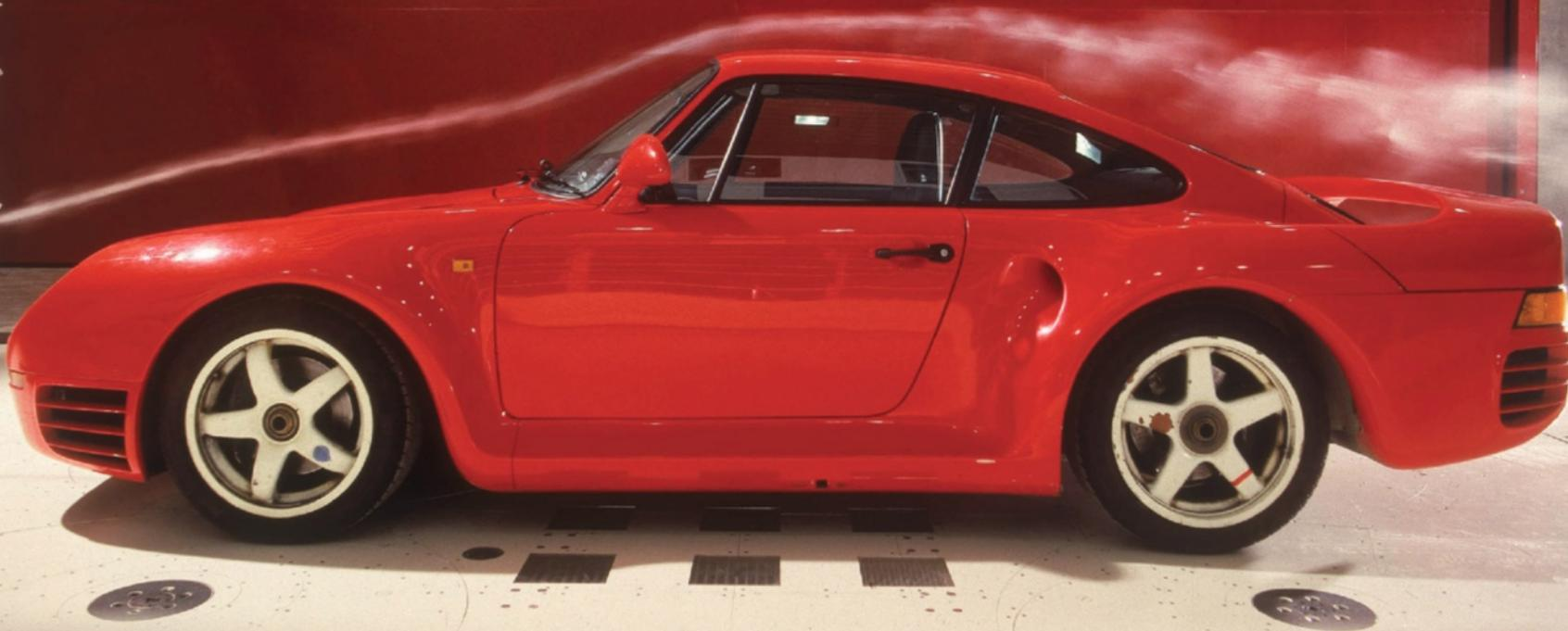
The Porsche Typ 959 underwent extensive aerodynamic testing in the new wind tunnel at Weissach in 1986, crucial for a supercar with a top speed of 186mph. This would be to the benefit of the 911 going forward, as we reveal next month
