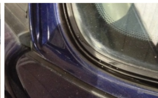
... while removing the outer trim could reveal water pooling in more serious cases
