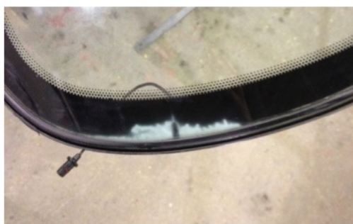
Check for signs of delaminating as a surefire warning that water has breached the windscreen...
