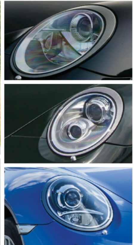
Lighting technology has advanced rapidly under the more traditional-looking 997 and 991 headlights, with LED surrounds now on PDLs Plus units (Targa, main pic)
