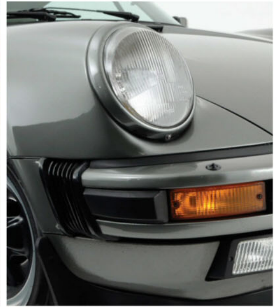
Early front light layout was unchanged for years before indicators moved into fenders for G program
