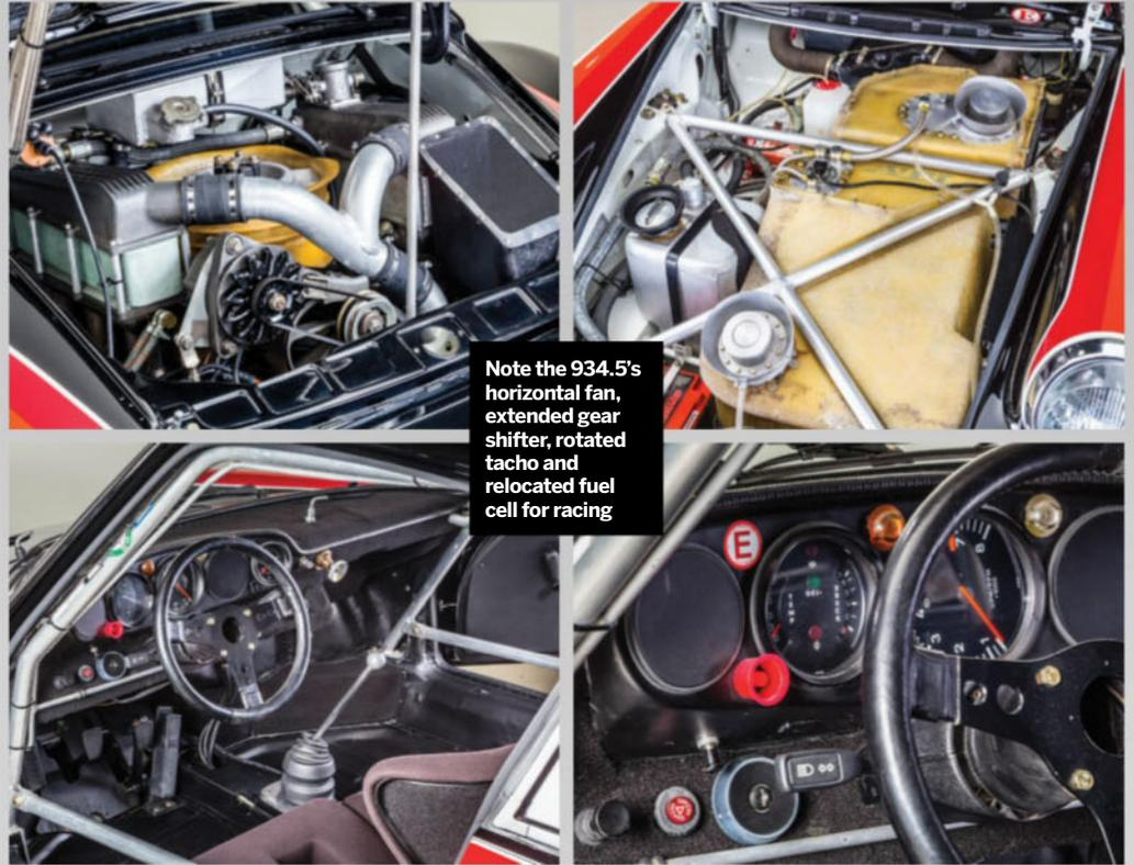
Note the 934.5's horizontal fan, extended gear shifter, rotated tacho and relocated fuel cell for racing
