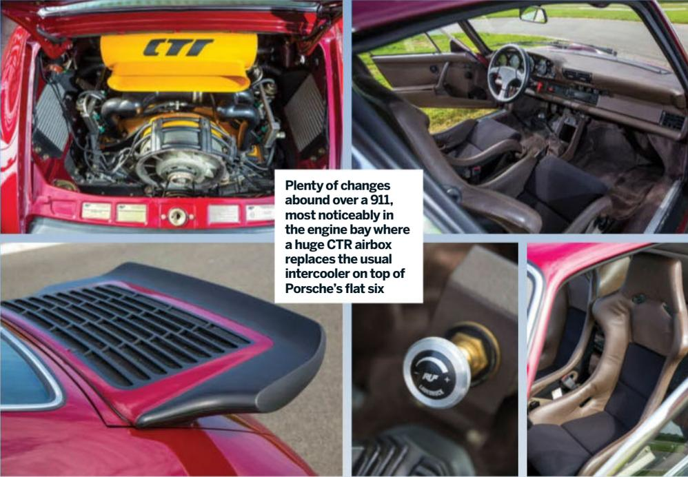
Plenty of changes abound over a 911, most noticeably in the engine bay where a huge CTR airbox replaces the usual intercooler on top of Porsche's flat six
