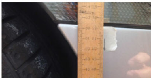
Above: The body of a 911 lifts when steering, with height measurements here when a wheel faces straight ahead (left) and turned (right)
