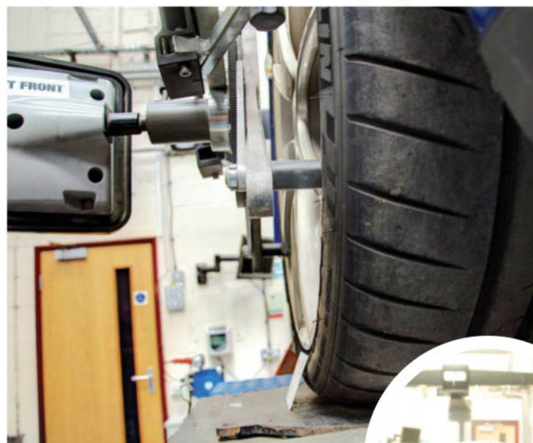
Above: The body of a 911 lifts when steering, with height measurements here when a wheel faces straight ahead (left) and turned (right)
