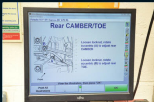
Above: Toe settings are usually set in tandem with camber
