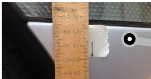
Above: The body of a 911 lifts when steering, with height measurements here when a wheel faces straight ahead (left) and turned (right)
