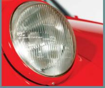
out, so it is recommended to check the bulbs at least every 20,000 kilometres for any signs of damage or dimming. A periodic review of the headlamps will prevent any nasty surprises, such as being unable to travel at night because of a burned-out bulb and subsequent poorly-lit road.
