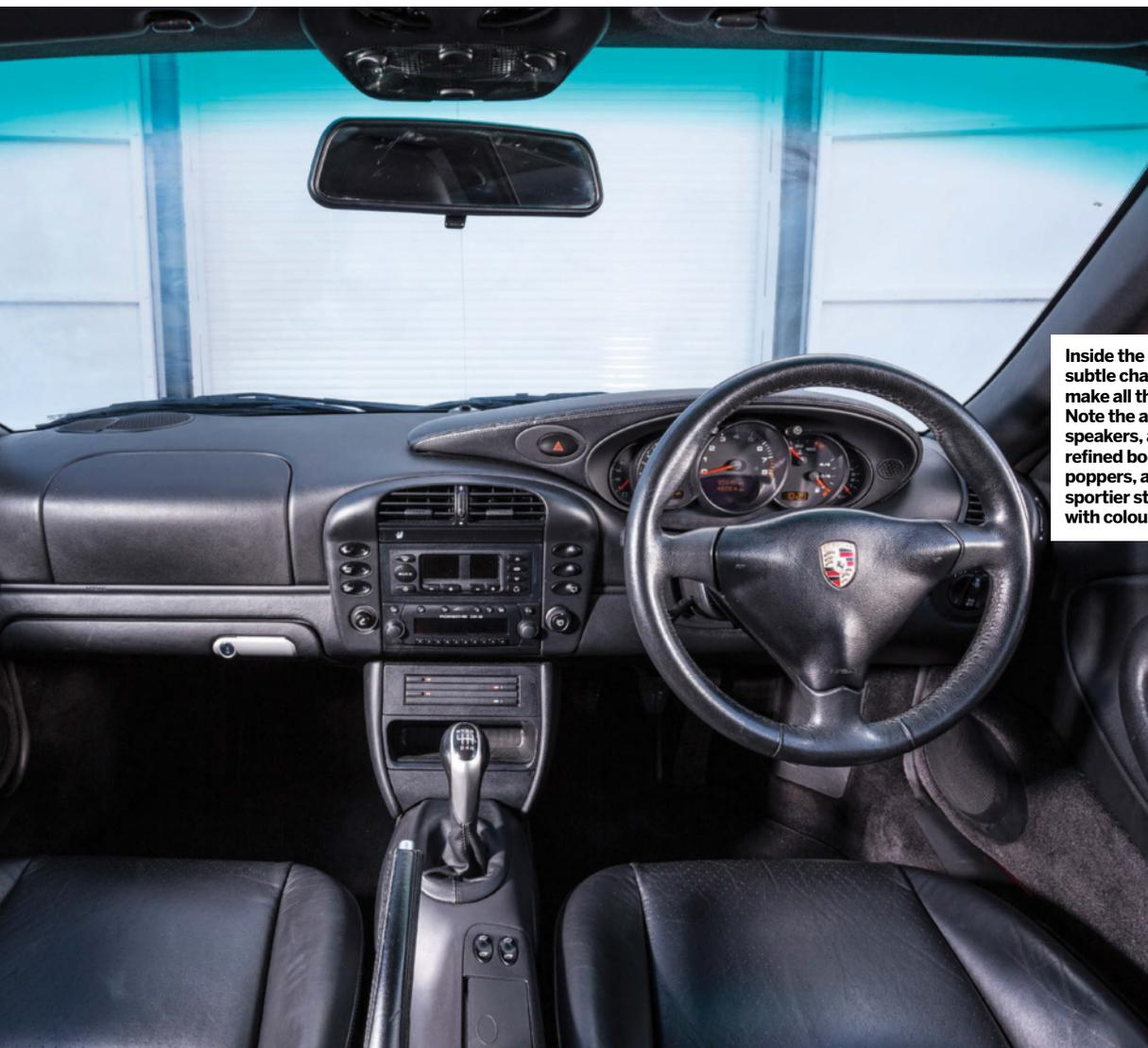
Inside the Gen2, it's the subtle changes that make all the difference. Note the addition of door speakers, a glove box, refined boot and decklid poppers, and a new, sportier steering wheel with coloured crest
