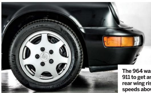
The 964 was the first 911 to get an active rear wing rising at speeds above 50mph; Design 90s were a new wheel style; on later cars, curved 'teardrop' exterior mirrors replaced 'elephant ear' items
