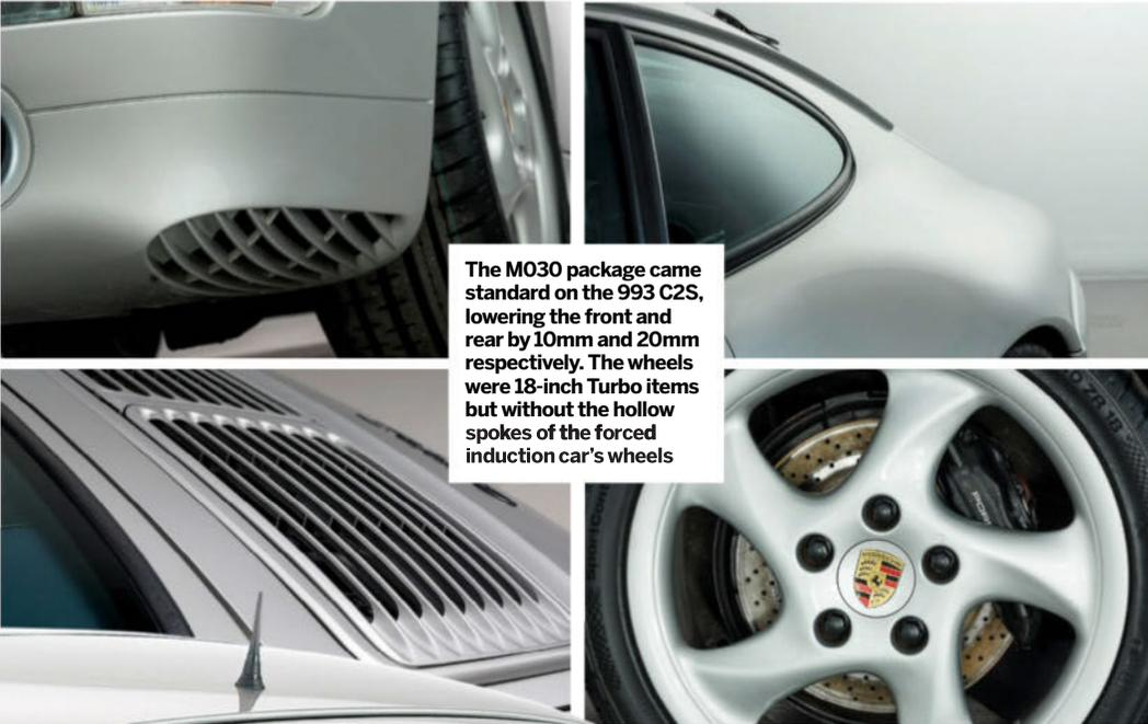
The M030 package came standard on the 993 C2S, lowering the front and rear by 10mm and 20mm respectively. The wheels were 18-inch Turbo items but without the hollow spokes of the forced induction car's wheels
