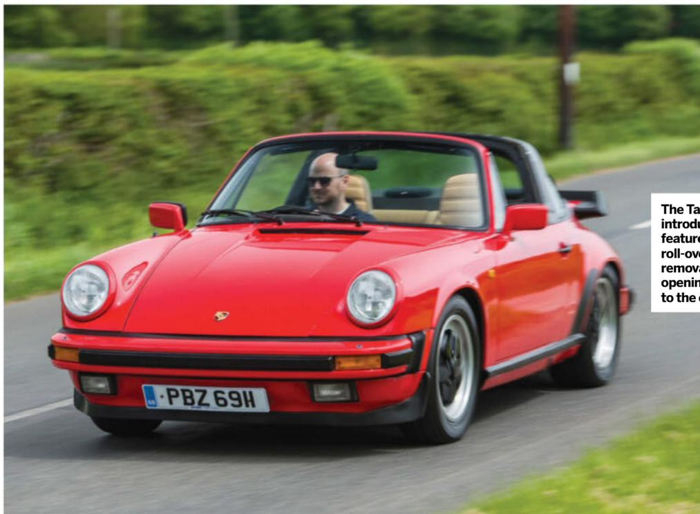
The Targa, first introduced in 1967, featured a full roll-over hoop and removable panel, opening the 911 up to the elements
