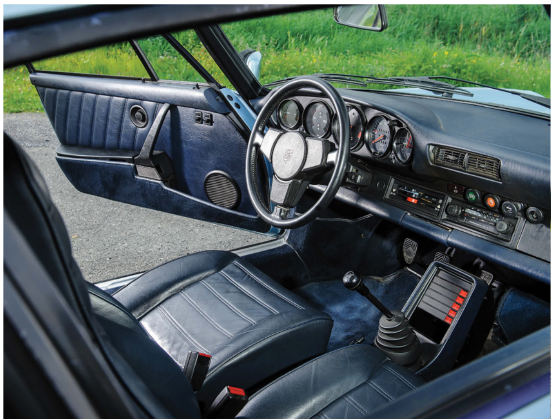
Right Factory SC interior complete with 915 five-speed gearbox, which had a longer fifth ratio for a slightly higher top speed
