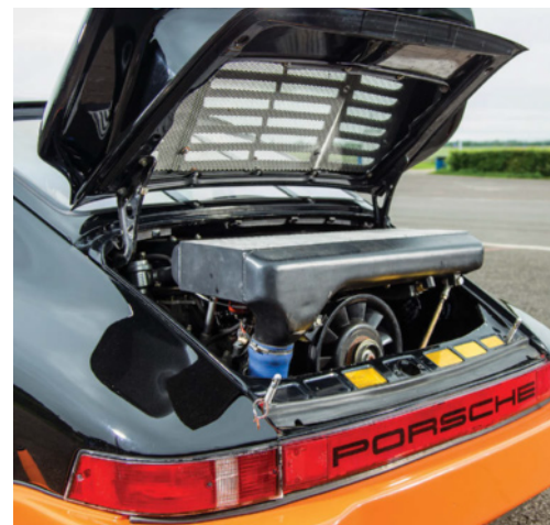
Above Huge 964 Turbo intercooler dominates the engine bay. Tweaks to the turbo and pistons raise the power output to over 400hp
