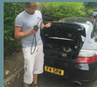
Porschacare fixed the problem quickly but, knowing the car well, pointed out that performance-wise it was driving like a standard Turbo, and not a remapped Turbo. I had thought it felt a little slower in recent weeks, but I had put that down to familiarity. It turns out that boost was capping out at 0.5 bar rather than 1.0 bar. We suspect an airflow sensor is on the way out; another issue that needs to be sorted but at least one we have diagnosed.
