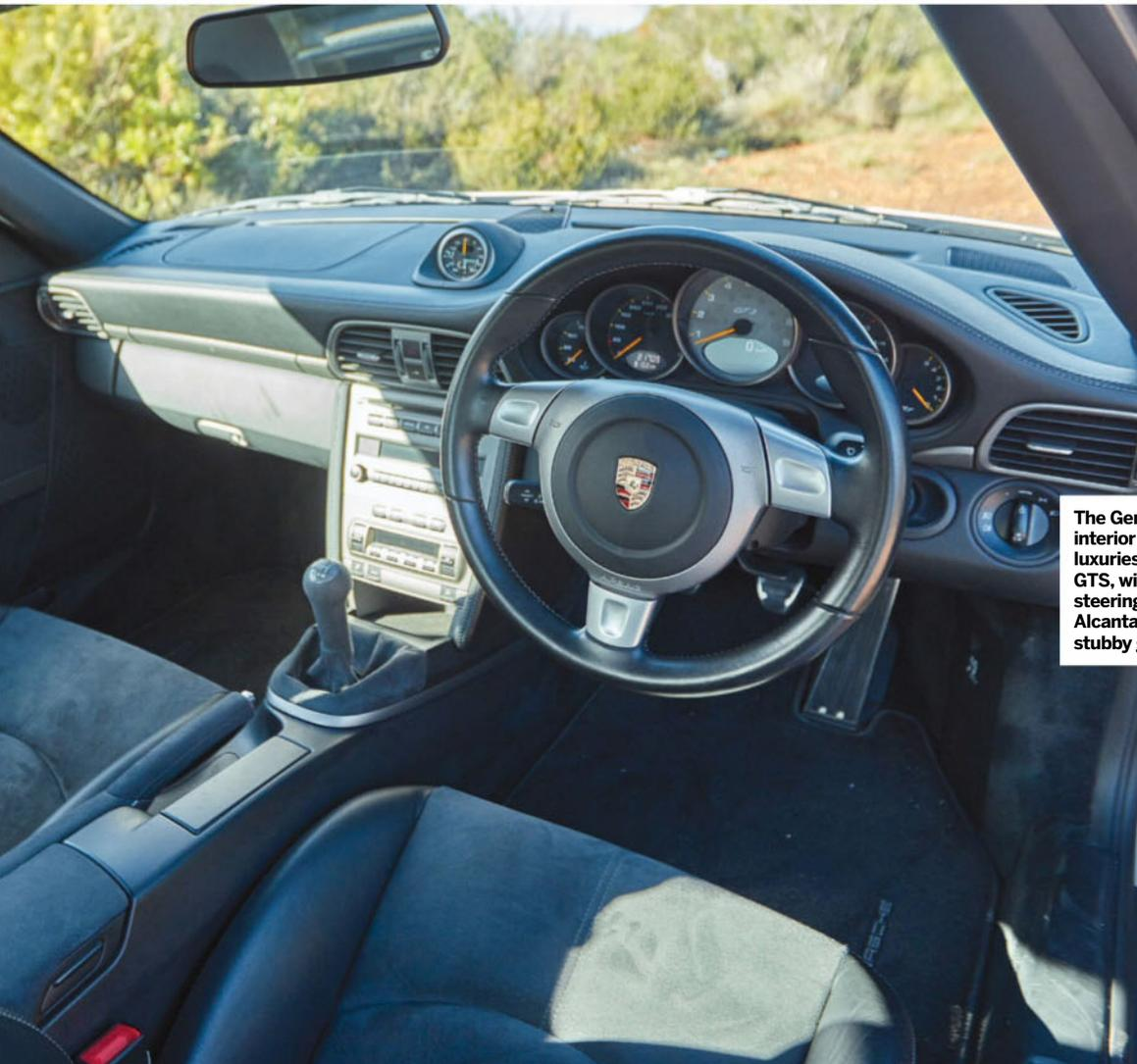
The Gen1 997 GT3's interior has fewer luxuries than the GTS, with a basic steering wheel and Alcantara-clad stubby gearlever
