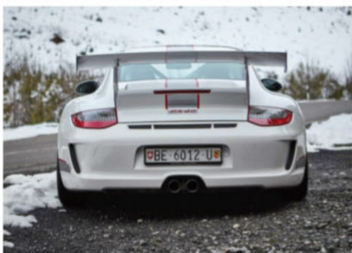
Above The purposeful huge rear wing of the 997 GT3 RS 4.0 is crafted from carbon fibre to reduce weight, as are the front fenders and the luggage compartment lid
