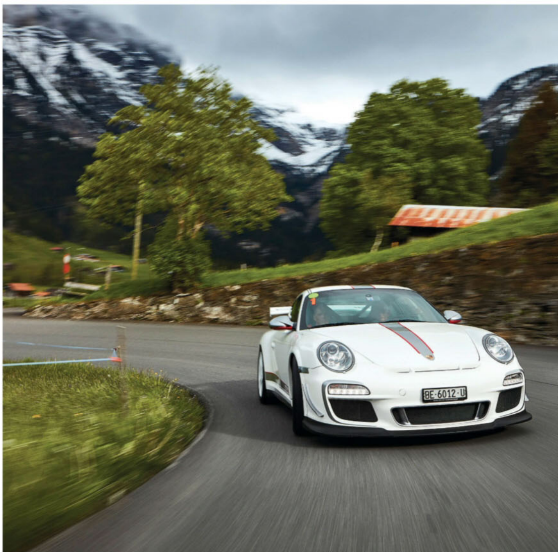
Above The purposeful huge rear wing of the 997 GT3 RS 4.0 is crafted from carbon fibre to reduce weight, as are the front fenders and the luggage compartment lid
