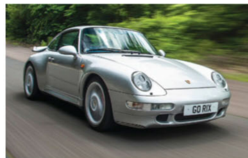
Above The 993 Turbo weighed an extra 30kg over its 964 predecessor but had power boosted by 48bhp
