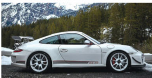
Above The purposeful huge rear wing of the 997 GT3 RS 4.0 is crafted from carbon fibre to reduce weight, as are the front fenders and the luggage compartment lid
