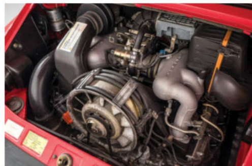
Above The 3.2's 930/20 flat six produced 231bhp and 284Nm of power and torque respectively
