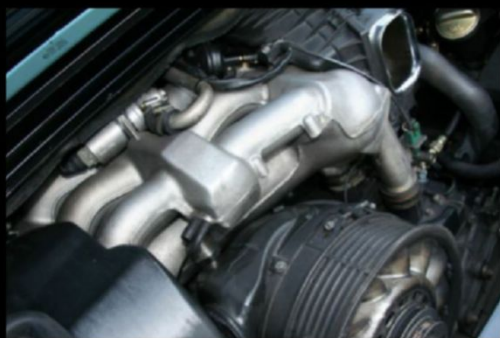
A 993 with Varioram is identifiable by magnesium pipes atop the flat six
