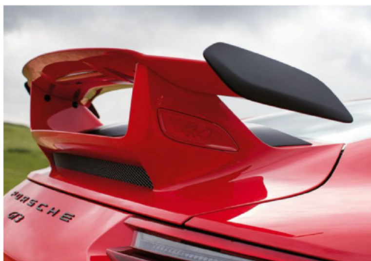
Above Fixed rear wing of 991.2 GT3 sits marginally higher up and further back than that of its predecessor. The result is 997 GT3 RS-matching levels of downforce
