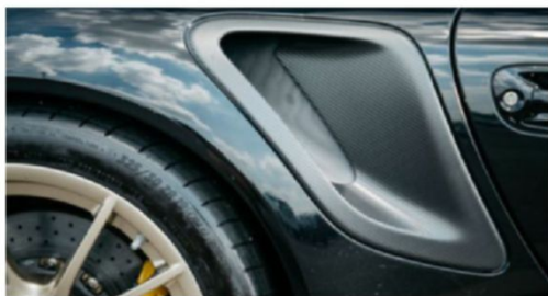
ABOVE Unpainted Carbon fibre details are all over the GT2 RS, including side air intakes, hot air exit vents and underside of front bonnet RIGHT Perspex screens aft of 'B' pillar help reduce overall mass
