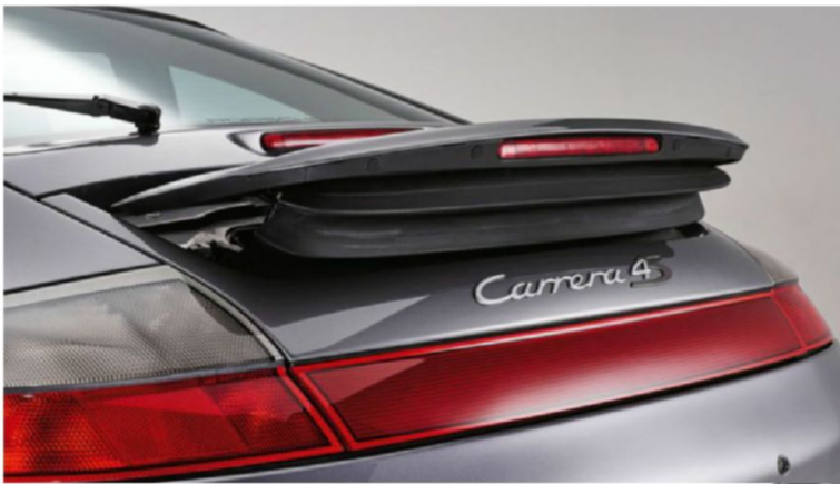
ABOVE AND RIGHT Rear spoiler automatically deploys at 75mph; Primitive PCM1 screen narrower than PCM2 found on later MY 2004 996s and onwards
