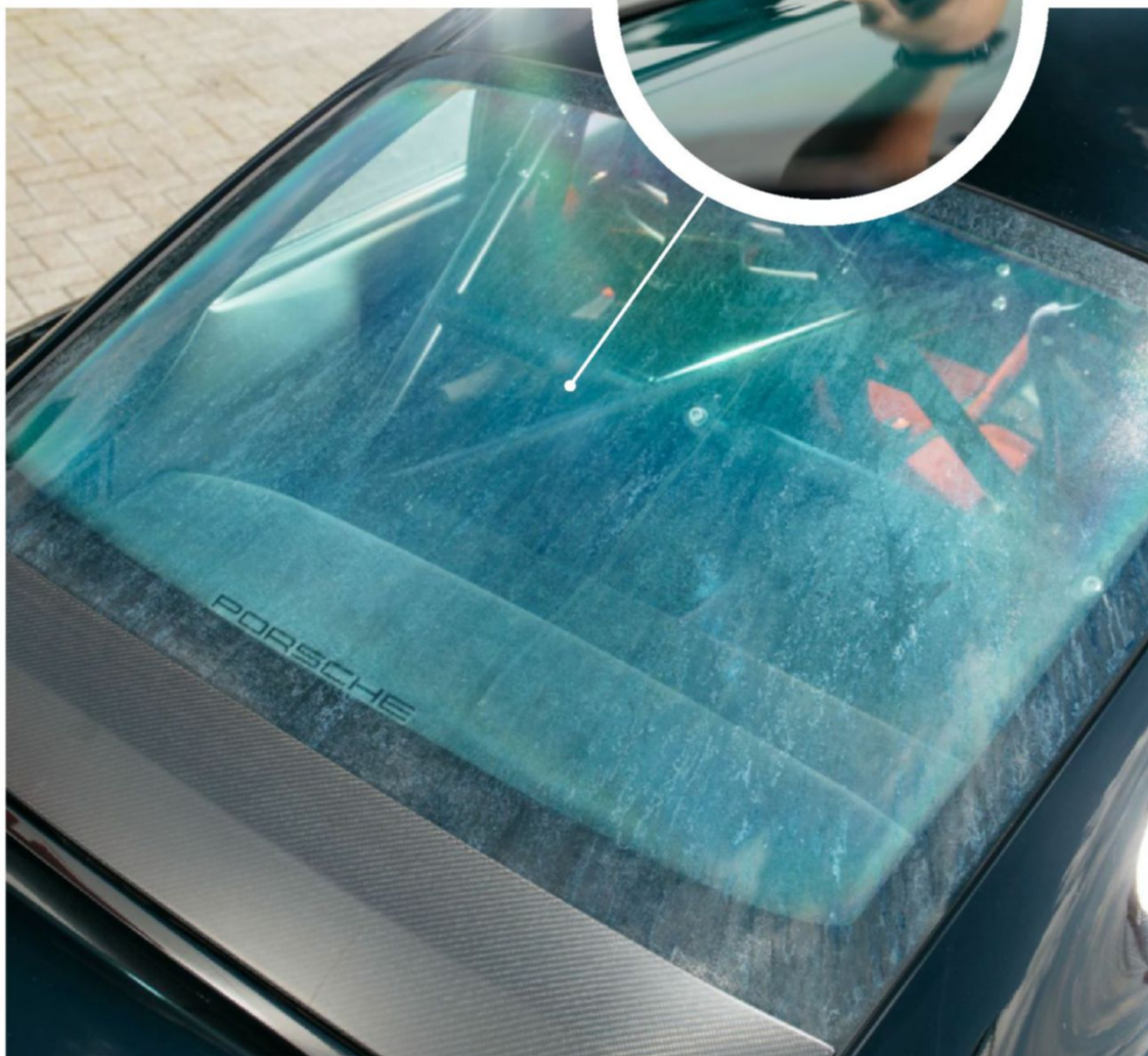
ABOVE Unpainted Carbon fibre details are all over the GT2 RS, including side air intakes, hot air exit vents and underside of front bonnet RIGHT Perspex screens aft of 'B' pillar help reduce overall mass
