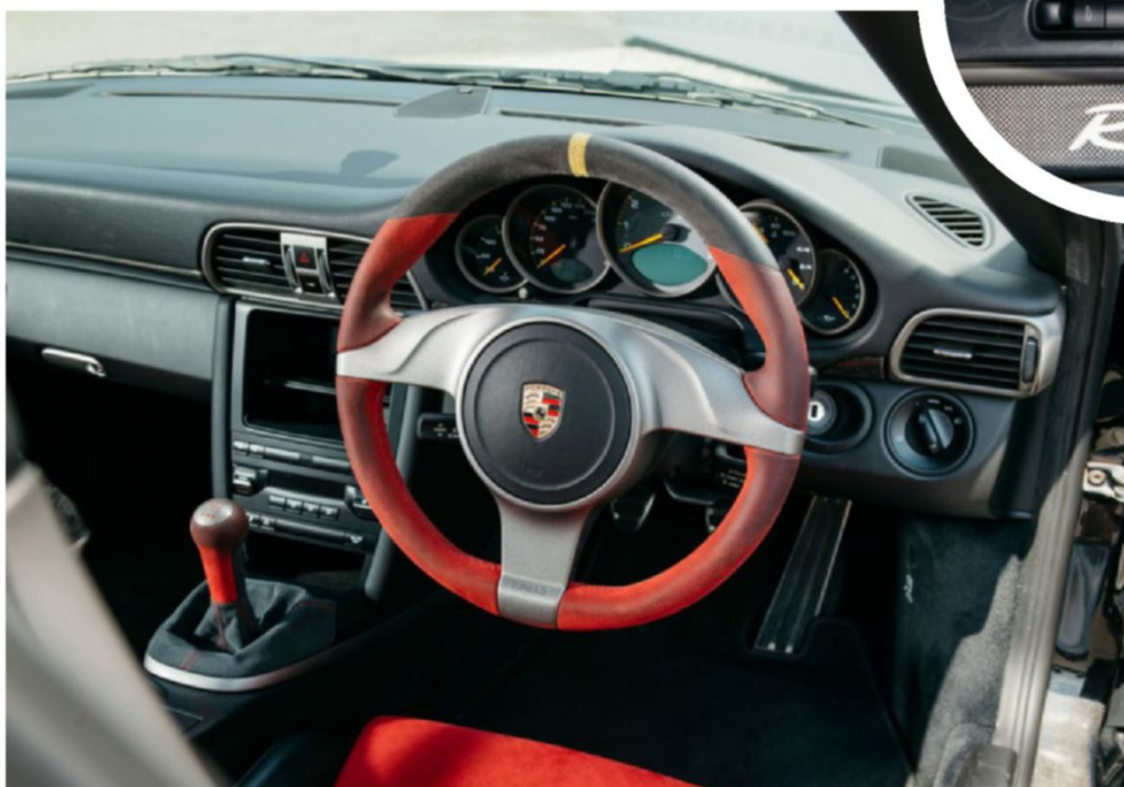
ABOVE Striking red alcantara in seat inserts and on steering wheel and shifter have become GT2 RS trademarks RIGHT PASM and stability/traction buttons occupy base of dash. 'Sport' button would be superfluous in the 997 GT2 RS
