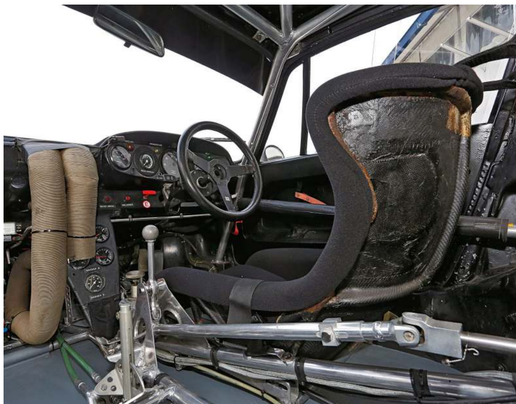
Seating position was moved to the right-hand-side on Moby Dick for better balance on predominantly clockwise circuits; gearbox oil cooler lay behind duct aft of driver's door
