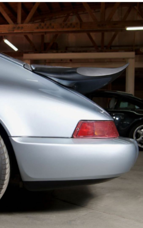
ABOVE AND LEFT The RSA's spec included a narrow-bodied C2 shell and engine with Turbo chassis and a basic interior comprising just four options. Whaletail was unique to the car for the era
