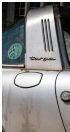
TOP AND BOTTOM Freshly rebuilt 2.4-litre 'T' engine currently powers the barn find while its original, matching numbers 2.4S engine is being rebuilt; External oil filler is a hallmark of MY1972 cars
