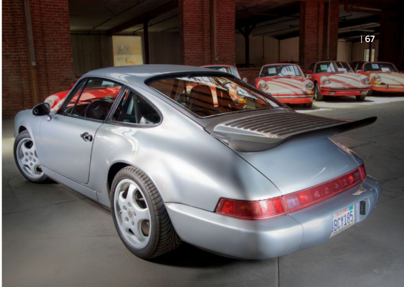
ABOVE AND LEFT The RSA's spec included a narrow-bodied C2 shell and engine with Turbo chassis and a basic interior comprising just four options. Whaletail was unique to the car for the era
