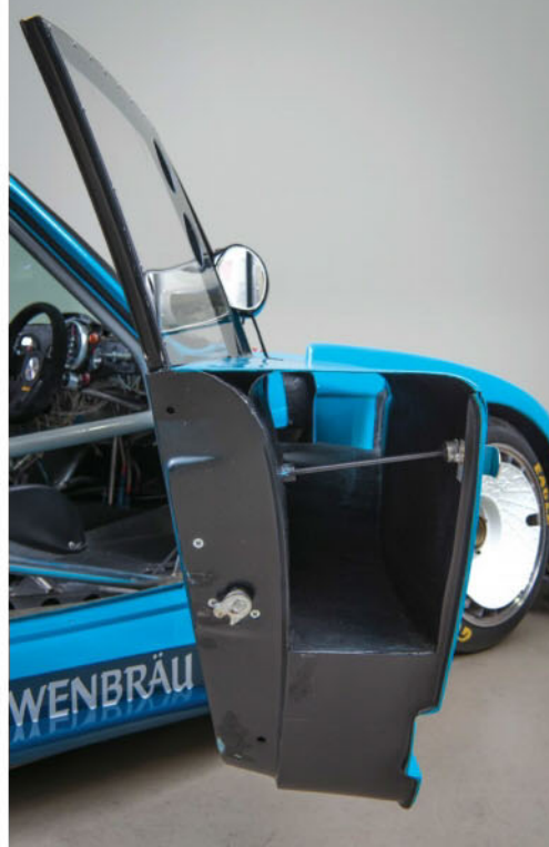
LEFT Cross-section of the K4's door shows notable body extension for channeling air affixed to original 930-esque panel
