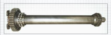
In every 911 engine up until the introduction of the 9A1 DFI unit, the crankshafts indirectly drive the camshafts via the intermediate shaft. Its use allows the speed of the timing chains to be reduced, increasing chain life. It's a set up that first appeared in the 547 flat four from the 356A Carrera.
