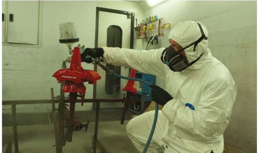
With that exhaustive prep work complete, it was time for paint. The colour of my Carrera 4S's 'Big Red' calipers is of course given away by their name, the special paint applied being resistant to heat by up to 300 degrees. Their appearance was gloss at first, yet this soon changed to a matte effect as we left the calipers in the oven to bake for ten minutes at 68 degrees.
