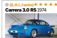
Updated version of the 1973 2.7 RS, complete with impact bumpers and Turbo-spec whaletail rear wing. Steel arches added by hand at the factory, with 917 brakes.
