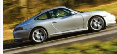
Facelifted with Turbo-style headlamps and revised front and rear bumpers, fitted with more powerful 3.6-litre engine and VarioCam Plus. Manual and Tiptronic boxes updated.
