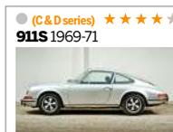
An upgrade in engine size gave the 911S 180bhp. Unlike the 911E, the S didn't gain improved low-down power and torque, so you had to keep the revs up for good power.
