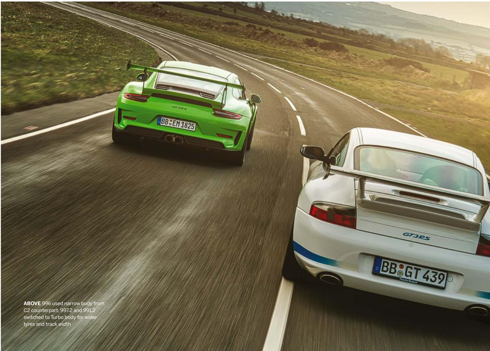
ABOVE 996 used narrow body from C2 counterpart, 997.2 and 991.2 switched to Turbo body for wider tyres and track width
