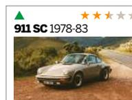
From 1978, the SC was the only normally aspirated 911. Developed from the Carrera 3.0, but produced less power. Upgraded Sport options.
