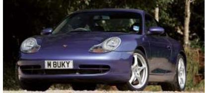
An all-new 911 with larger, restyled bodywork and a water-cooled engine. Interior was redesigned in order to enable better ergonomic efficiency and more room.
