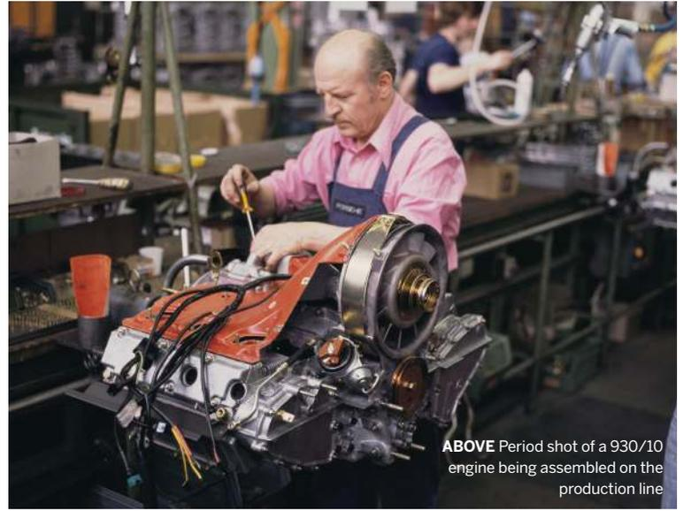
ABOVE Period shot of a 930/10 engine being assembled on the production line
