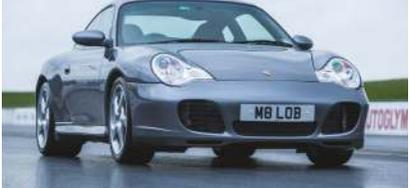
Basically a C4 featuring a Turbo bodysell, without rear air intakes, but with a full-width rear reflector panel. Suspension and brakes were similar to the Turbo spec.
