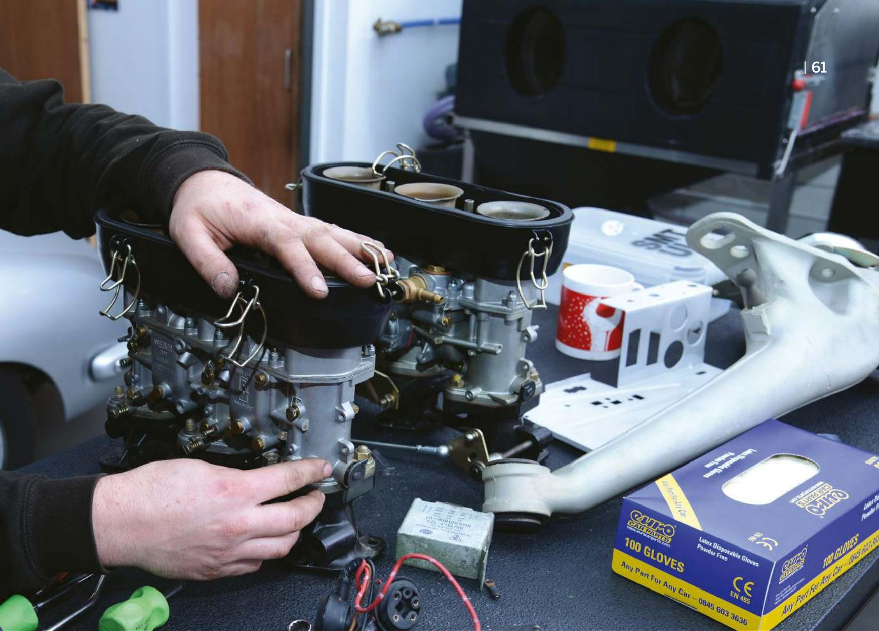
for induction after just 18 months of 911 production, and Weber remained the mainstay until emissions regulations dictated the move to Mechanical Fuel Injection. The Triple Weber system is not unique to Porsche's 911. The Italian company at that time probably supplied 99 per cent of the performance cars in the world with either single-, double- or triple-choke systems. Triple Webers can be found on Lamborghini, Ferrari and Maserati of the time.
