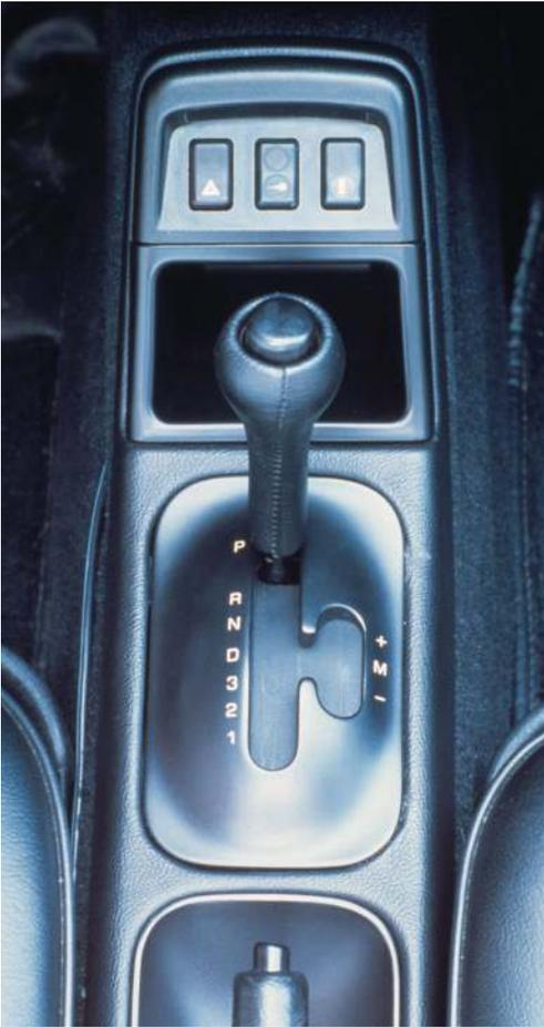
**ABOVE** Four-speed Tiptronic gearbox debuts on the 911 for the first time with the 964
