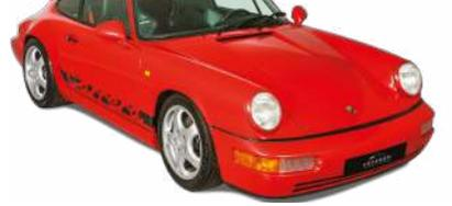
120kg saved by deleting 'luxuries' and fitting magnesium Cup wheels. Power was boosted by 10bhp, suspension lowered by 40mm and updated, as were brakes.
