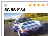
True homologation special built so that Porsche could go Group B rallying. Six Rothmans cars used fibre glass front wings and lid. Tuned 3.0-litre engine had its basis in 930's crankcase.
