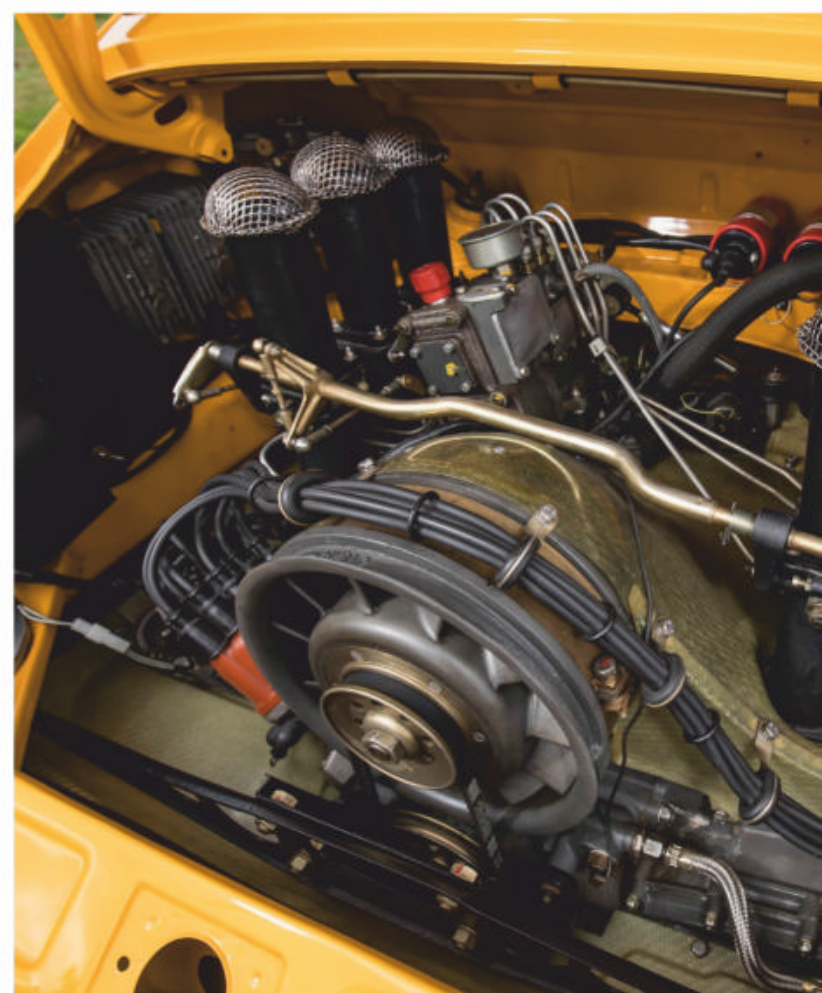
ABOVE RSR's flat six was upgraded to twin plug specification as part of an overhaul resulting in a 98hp boost over a 2.7 RS
