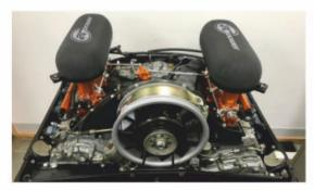
Take the diminutive proportions of a classic 911 and pop a tuned Mezger in the back. 3.5litres, AT power throttle bodies, converted to coil on plug, all managed by MOTEC M150 control. One can only imagine the serrated throttle response and banshee wail this produces in the back of a light, narrow body classic 911. Dreamy.
