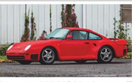
337 \* \* \* \* Production numbers Issue featured **Engine capacity** 2.850cc Compression ratio 8.3:1 Maximum power 450hp @ 6,500rpm 500Nm @ 5,000rpm 0-60mph 196mph Top speed 4,260mm Length Width 1,840mm Weight Wheels & tyres F 8x17 inch; 235/45/ZR17 1,450kg R 9x17 inch; 255/40/ZR17
